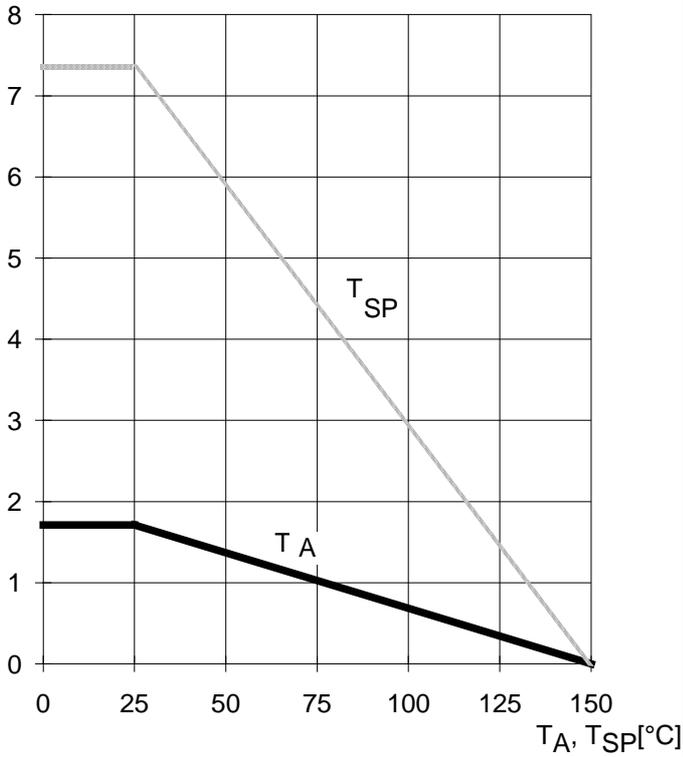
Typ. on state resistance (V<sub>bb</sub>- pin to OUT pin)
