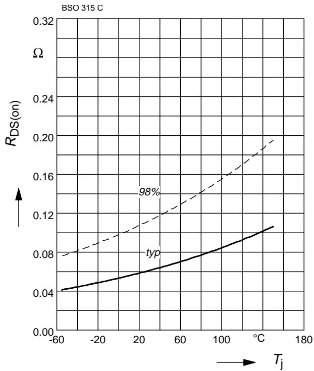
**Drain-source on-resistance (P-Ch.)**
