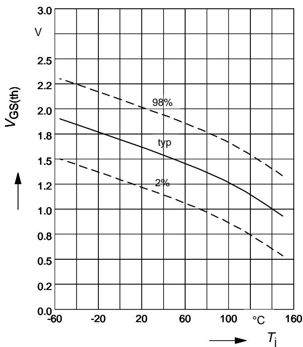
**Gate threshold voltage (P-Ch.)**
