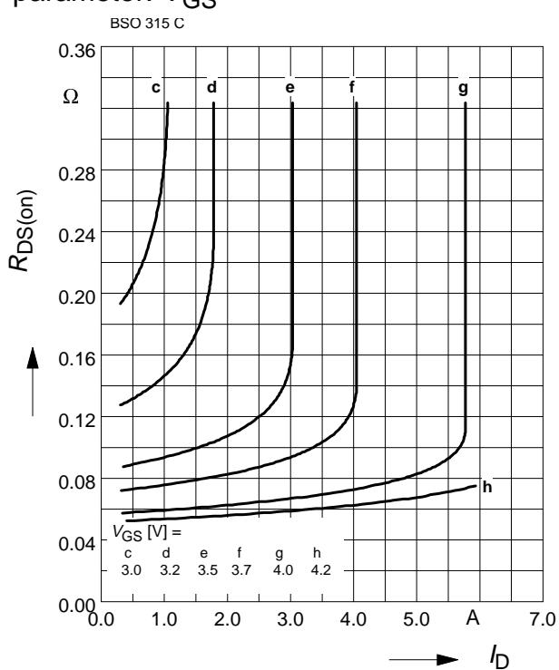
**Typ. drain-source-on-resistance (P-Ch.)**
