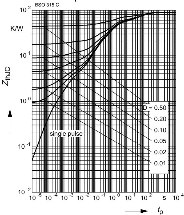
**Transient thermal impedance (P-Ch.)**
