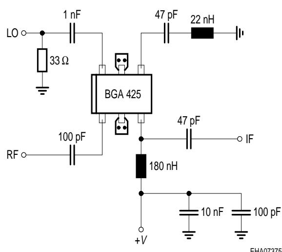
Note: 1) Large-value capacitors should be connected from pin 6 to ground right at the device to provide a low impedance path! (appl. 1)
