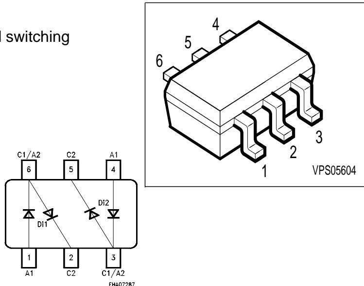
**ESD:** Electrostatic discharge sensitive device, observe handling precautions!
