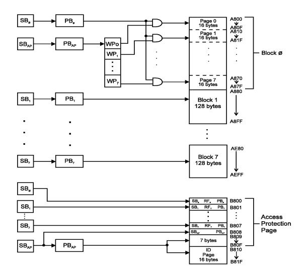
There is no individual page Write Protection for any other block other than block 0 within the device. Within the remaining blocks on the chip, access permissions are controlled on a block basis (PB or RF bits) or full chip basis (WP pin) only.
