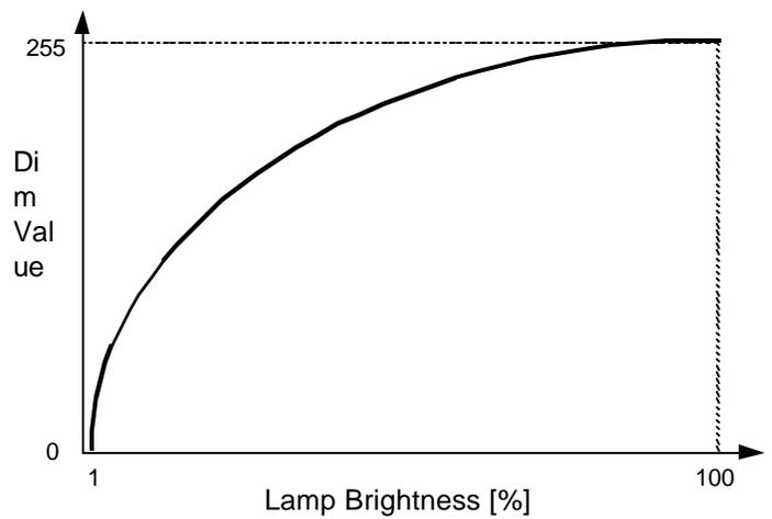
Figure 5, DALI logarithmic dimming curve with 256 brightness levels
