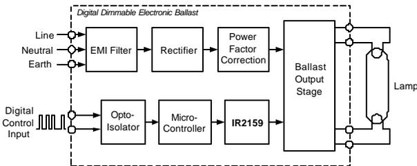
Figure 4, Digital dimming solution using the IR2159 Dimming IC.
