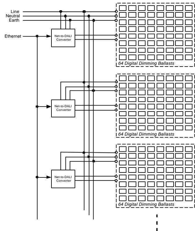
Figure 1, Typical digital dimming system.
