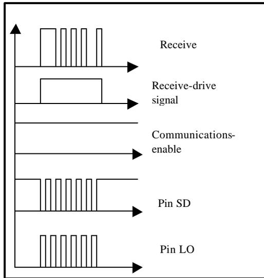
Figure 13, Communication Signals between micro-controller/DALI
