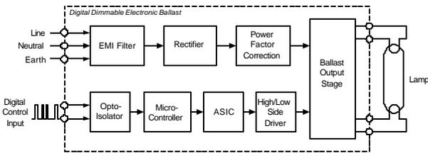
Figure 3, Typical digital dimming ASIC solution.
