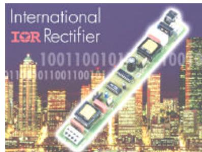
Figure 6, IRPLDIM2: Digitally Addressable DALI Dimming Ballast
