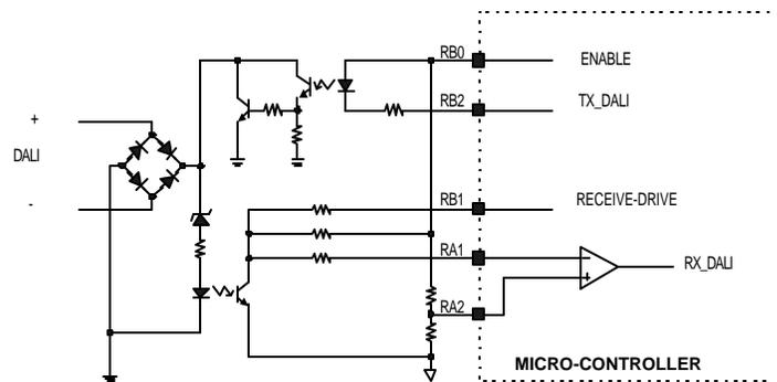
Figure 11, DALI/ Micro-controller communication.
