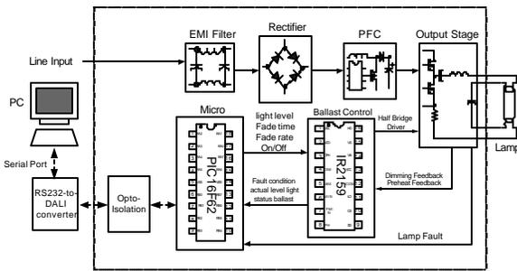
Figure 8, IRPLDIM2 Digitally Addressable Dimming Ballast.
