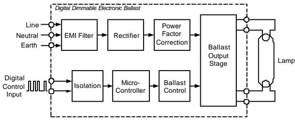
Figure 2, Digital dimming ballast block diagram.
