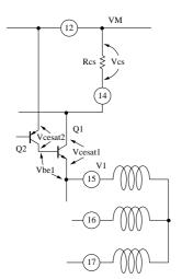
The V15 voltage of upper transistor block is given as follows:
