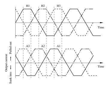
When EC > ECR, the pulling-out and sinking-into of the output current is just reversed from those shown in the above figure, and the motor rotation direction is reversed.
