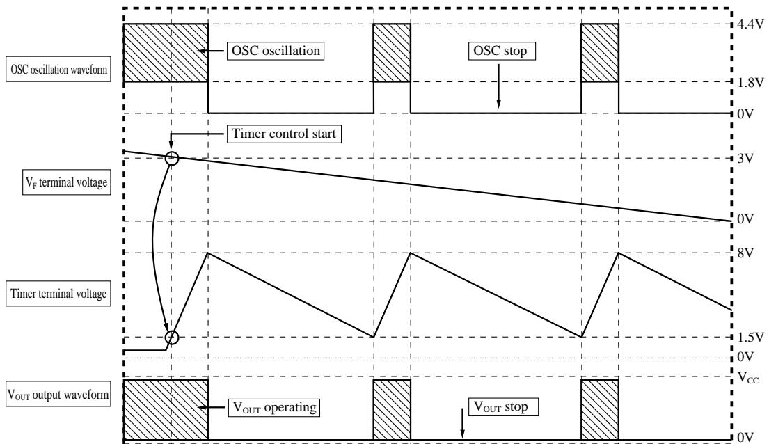
Note 2) The  $T_{OFF(max)}$  control and timer control work under current-limited operation ( $CLM+ \geq 0.2V$ ,  $CLM- \leq -0.2V$ )
