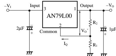
$$|V_O| = V_O' \left( 1 + \frac{R_1}{R_2} \right) + I_Q R_1$$
