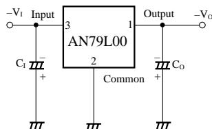
C<sub>I</sub> is connected when the input line is long. 2μF
