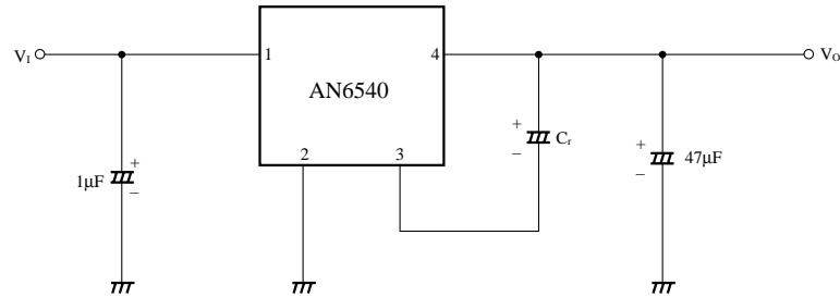
Note) Choose the oscillation control capacitor 47μF which has a small capacitance reduction even at a low temperature. For example, use the tantalum capacitor.
