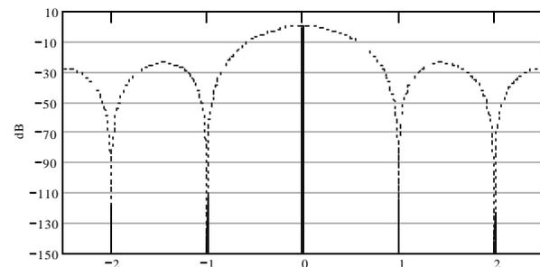
The table below lists maximum bandwidth that will be rejected to various levels for CIC2 interpolation factors from 1 to 32. The example above corresponds to the listing in the -110dB column and the  $L_{CIC2}=5$  row. It is worth noting here that the rejection of the CIC2 improves as the interpolation factor increases.
