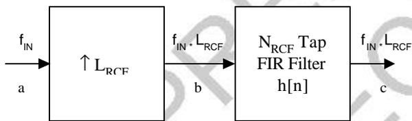
The difference equation for the diagram above is written below, where  $h[n]$  is the RCF impulse response,  $b[n]$  is the interpolated input sample sequence at point 'b' in the diagram above, and  $c[n]$  is the output sample sequence at point 'c' in the diagram above.
