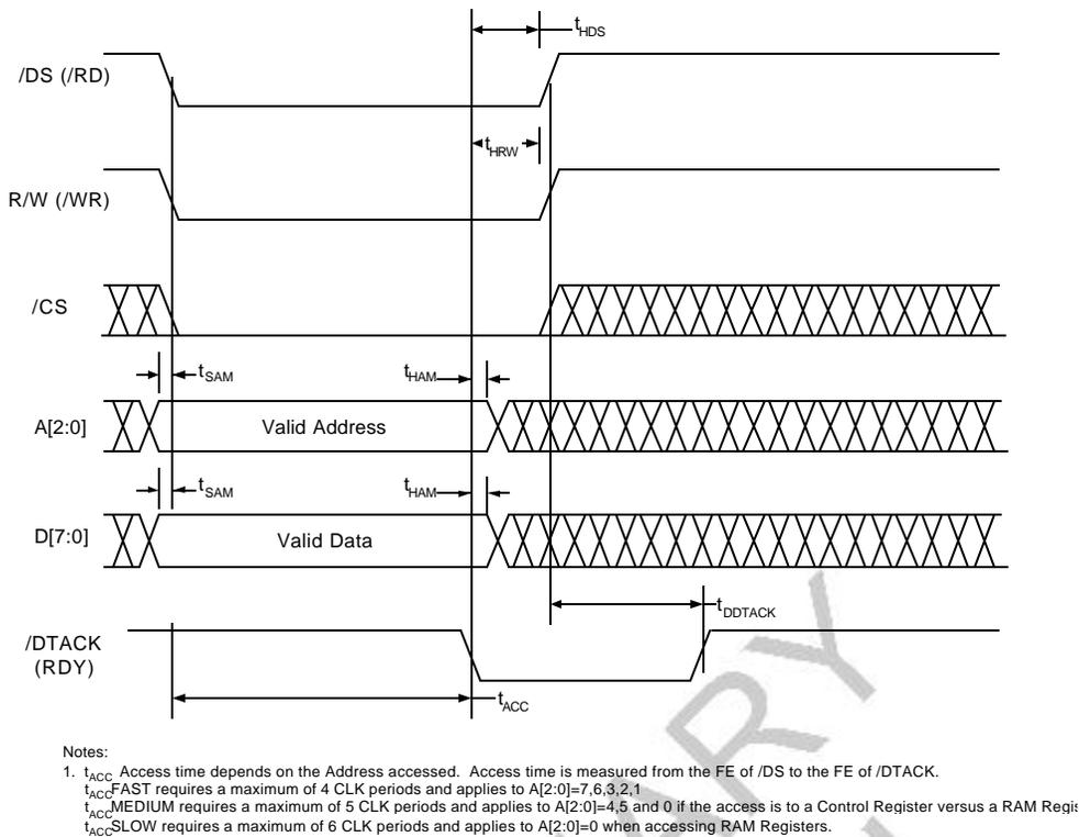
Figure X. MNM MicroPort Write Timing Requirements.
