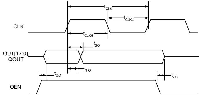
Figure X. Parallel Output Switching Characteristics.
