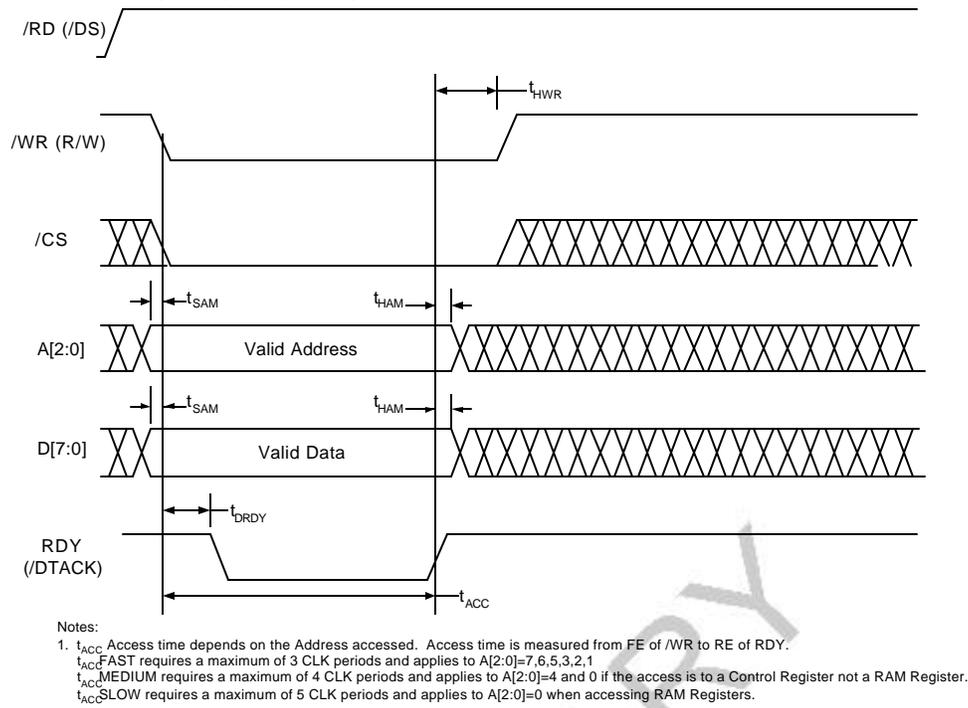
Figure X. INM MicroPort Write Timing Requirements.
