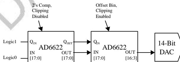
Figure XX. Cascade Operation of two AD6622s.
