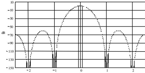
The table below lists maximum bandwidth that will be rejected to various levels for CIC5 interpolation factors from 1 to 32. The example above corresponds to the listing in the -110dB column and the  $L_{CIC5}=5$  row. It is worth noting here that the rejection of the CIC5 improves as the interpolation factor increases.
