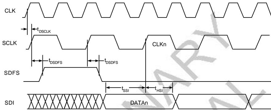
Figure X. Serial Port Switching Characteristics.
