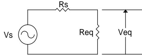
**Figure 4.. Equivalent Simplified Schematic**
