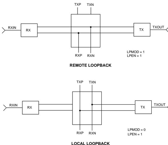
Figure 2. Loopback Configurations
