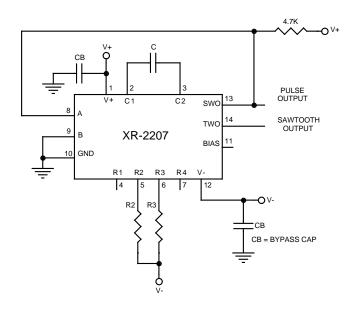
Figure 18. Duty Cycle Control
