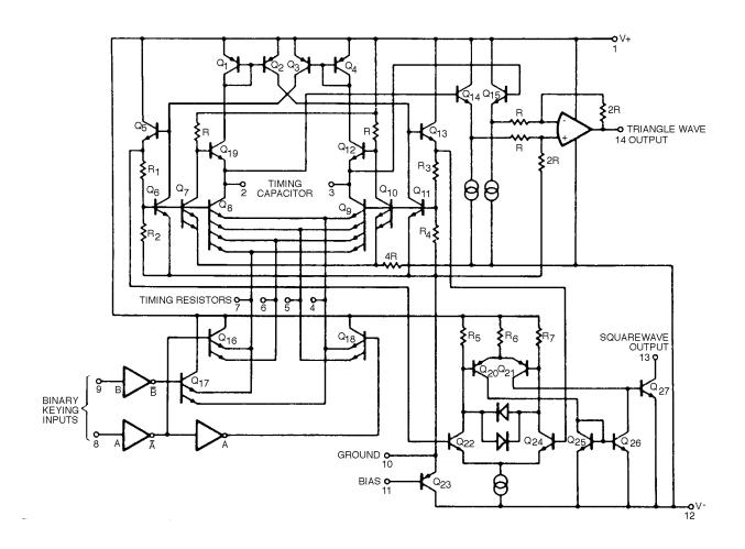
Figure 2. Equivalent Schematic Diagram
