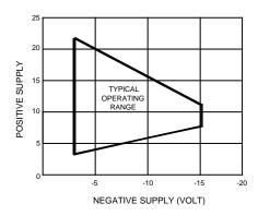
Figure 5. Operating Range For Unequal Split Supply Voltages
