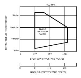
Figure 8. Recommended Timing Resistor Value vs. Power Supply Voltage\*
