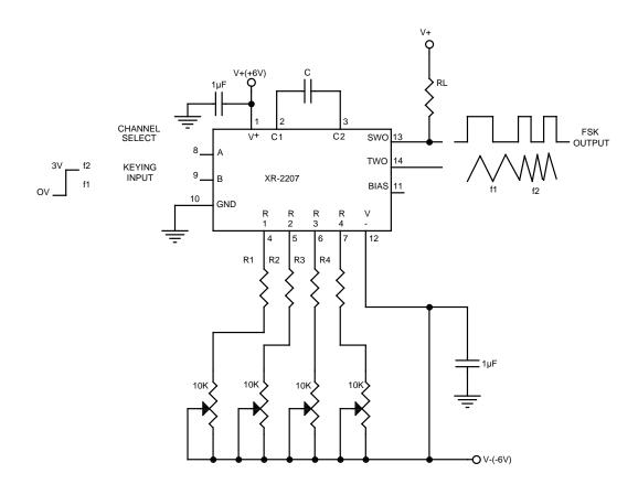
Figure 20. Multi-Channel FSK Generation
