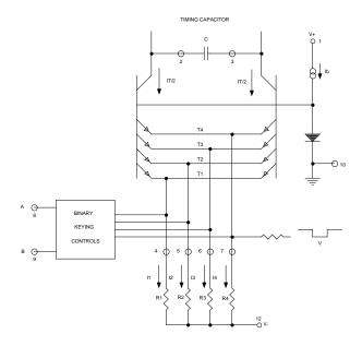
Figure 12. Simplified Schematic of Frequency Control Mechanism
