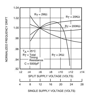
Figure 10. Frequency Drift vs. Supply Voltage
