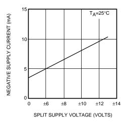
Figure 7. Negative Supply Current, I<sup>-</sup> (Measured at Pin 12) vs. Supply Voltage
