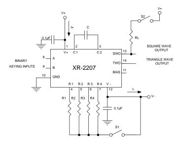
Figure 4. Test Circuit For Split Supply Operation
