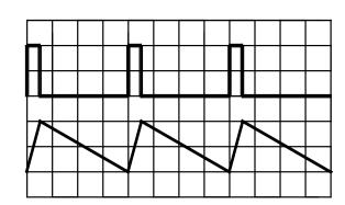
**B - Pulse and Sawtooth Outputs**
