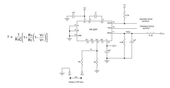
Figure 17. Frequency Sweep Operation, Single Supply
