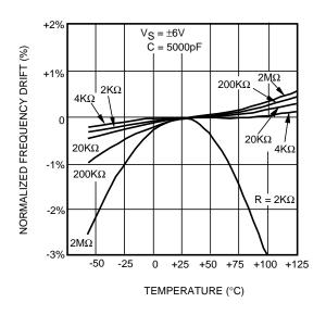
Figure 11. Normalized Frequency Drift with Temperature
