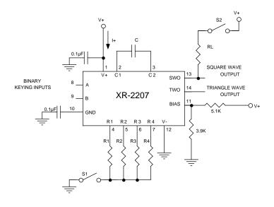
Figure 3. Test Circuit For Single Supply Operation
