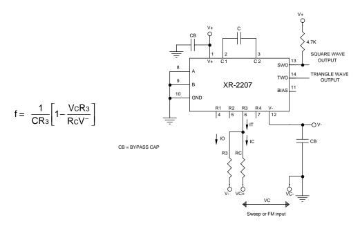
Figure 15. Frequency Sweep Operation, Split Supply
