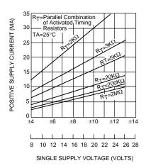
Figure 6. Positive Supply Current, I<sup>+</sup> (Measured at Pin 1) vs. Supply Voltage
