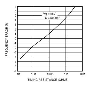
Figure 9. Frequency Accuracy vs. Timing Resistance
