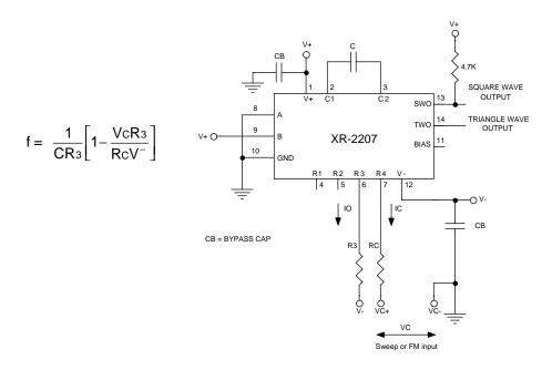
Figure 16. Alternate Frequency Sweep Operation, Split Supply
