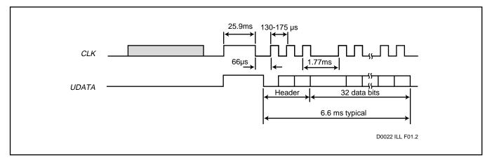
Decoder outputs are always preceded by a 25.9 ms header pulse on both CLK and UDATA. The user's controller will normally keep UDATA low and sample CLK every 25 ms or less. If it finds CLK high, UDATA will be configured as an input and sampled. If UDATA is found high, it is an indication of a pending decoder output. If it is found low, UDATA must immediately be pulled low again and the controller may proceed with other duties, sampling again within 25ms.
