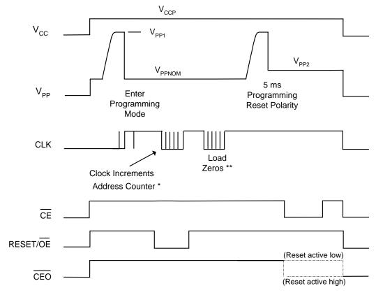
\* Number of Clocks for the Device Reset Polarity Location
