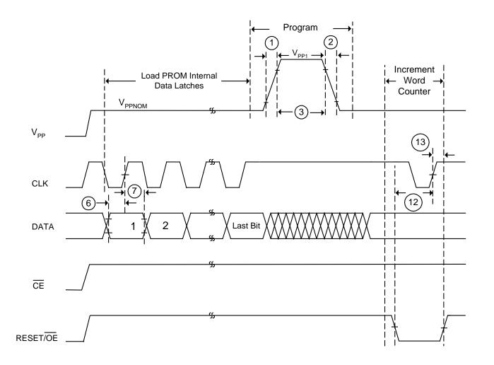
Figure 4. Details Of The Programming Cycle
