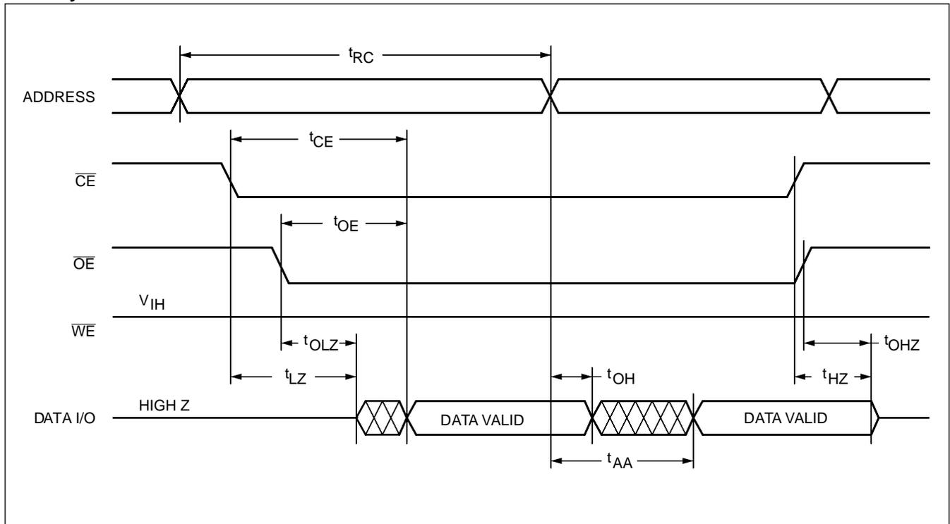
**Notes:** (3)  $t_{LZ}$  min.,  $t_{HZ}$ ,  $t_{OLZ}$  min., and  $t_{OHZ}$  are periodically sampled and not 100% tested.  $t_{HZ}$  max. and  $t_{OHZ}$  max. are measured, with  $C_L = 5\text{pF}$ , from the point when  $\overline{CE}$  or  $\overline{OE}$  return HIGH (whichever occurs first) to the time when the outputs are no longer driven.
