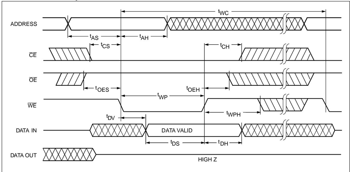
**Notes:** (4)  $t_{WC}$  is the minimum cycle time to be allowed from the system perspective unless polling techniques are used. It is the maximum time the device requires to complete internal write operation.
