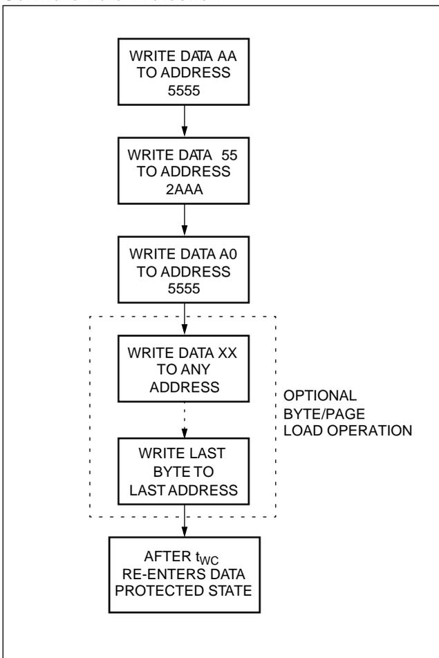
Regardless of whether the device has previously been protected or not, once the software data protection algorithm is used and data has been written, the X28C010 will automatically disable further writes unless another command is issued to cancel it. If no further commands are issued the X28C010 will be write protected during power-down and after any subsequent power-up. The state of  $A_{15}$  and  $A_{16}$  while executing the algorithm is don't care.
