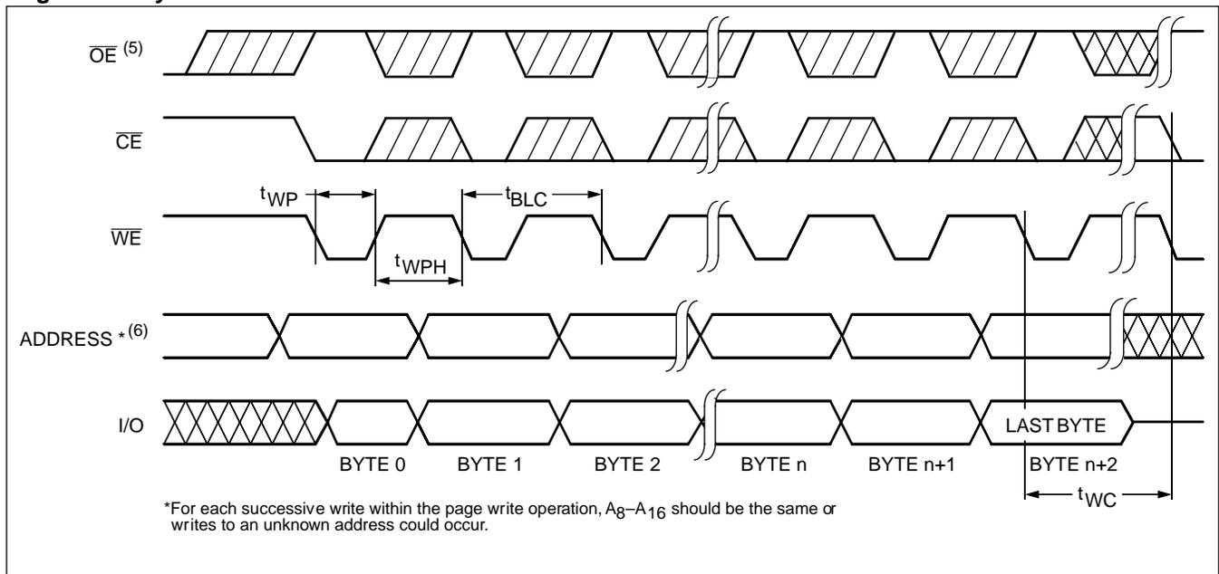
**Notes:** (5) Between successive byte writes within a page write operation,  $\overline{OE}$  can be strobed LOW: e.g. this can be done with  $\overline{CE}$  and  $\overline{WE}$  HIGH to fetch data from another memory device within the system for the next write; or with  $\overline{WE}$  HIGH and  $\overline{CE}$  LOW effectively performing a polling operation.
