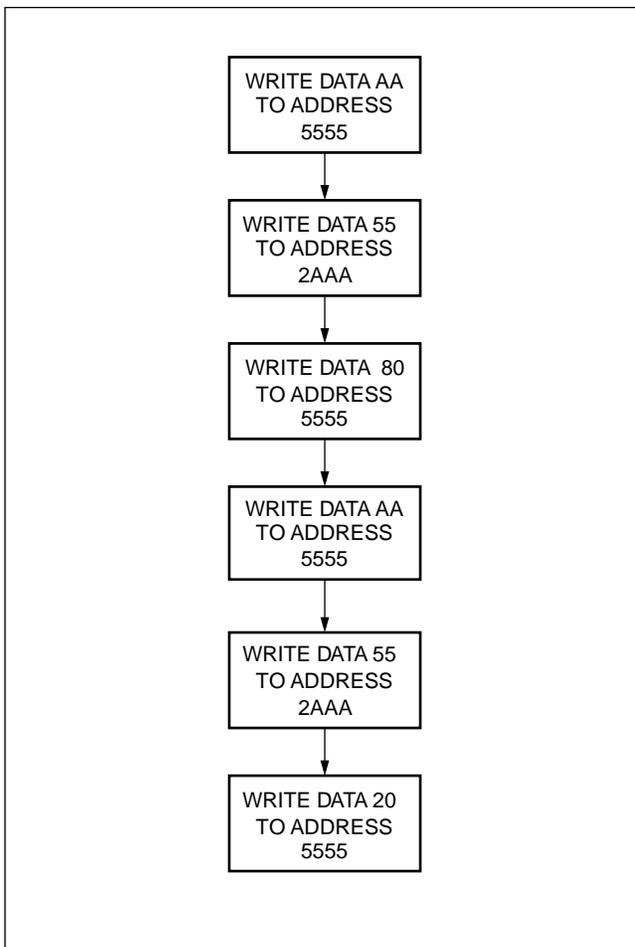
In the event the user wants to deactivate the software data protection feature for testing or reprogramming in an E<sup>2</sup>PROM programmer, the following six step algorithm will reset the internal protection circuit. After  $t_{WC}$ , the X28C010 will be in standard operating mode.
