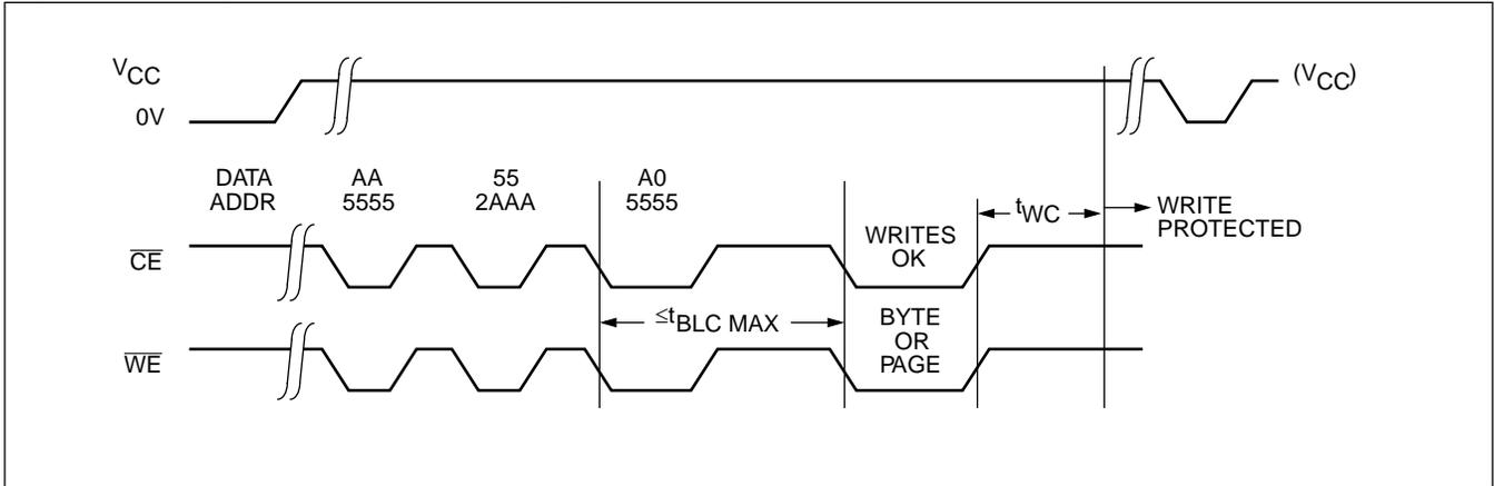
**Figure 7. Write Sequence for Software Data Protection**
