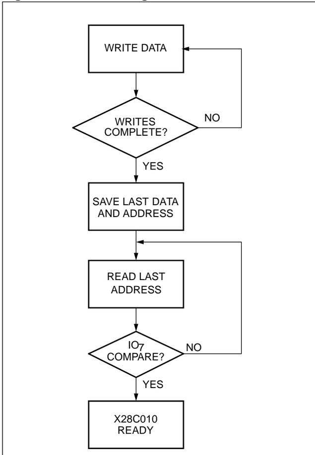
DATA Polling can effectively halve the time for writing to the X28C010. The timing diagram in Figure 2 illustrates the sequence of events on the bus. The software flow diagram in Figure 3 illustrates one method of implementing the routine.
