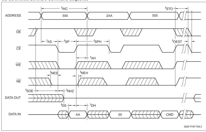
$\textbf{Note:} \quad \text{(6)} \ \, \text{The Store Pulse Width (t$_{SP}$) is a minimum time that $\overline{\text{NE}}$, $\overline{\text{WE}}$ and $\overline{\text{CE}}$ must be LOW simultaneously.}$
