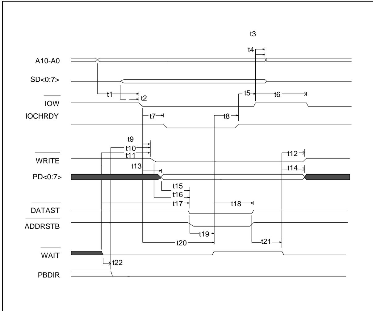
**13.3.4 EPP Data or Address Read Cycle (EPP Version 1.7)**
