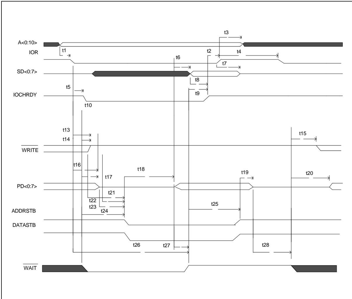
**13.3.5 EPP Data or Address Write Cycle (EPP Version 1.7)**
