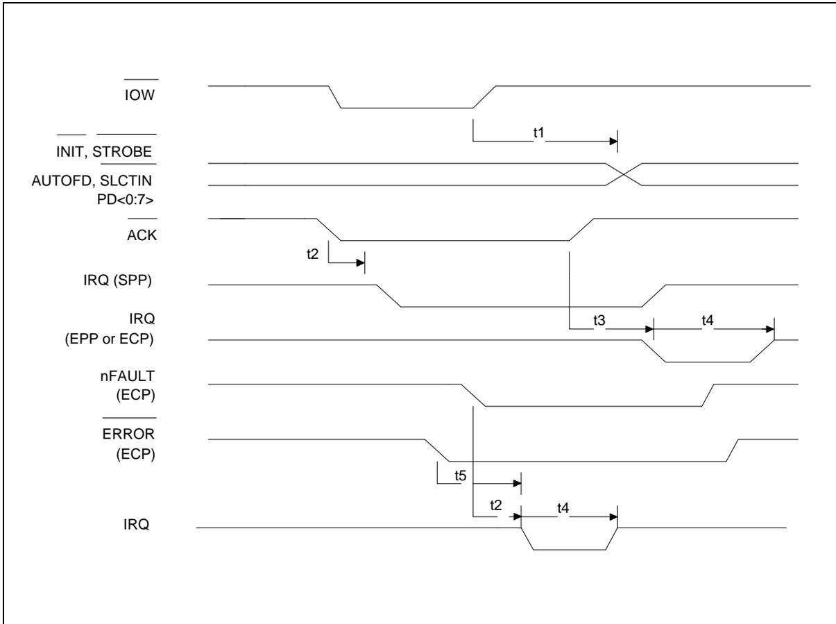
**13.3.2 EPP Data or Address Read Cycle (EPP Version 1.9)**
