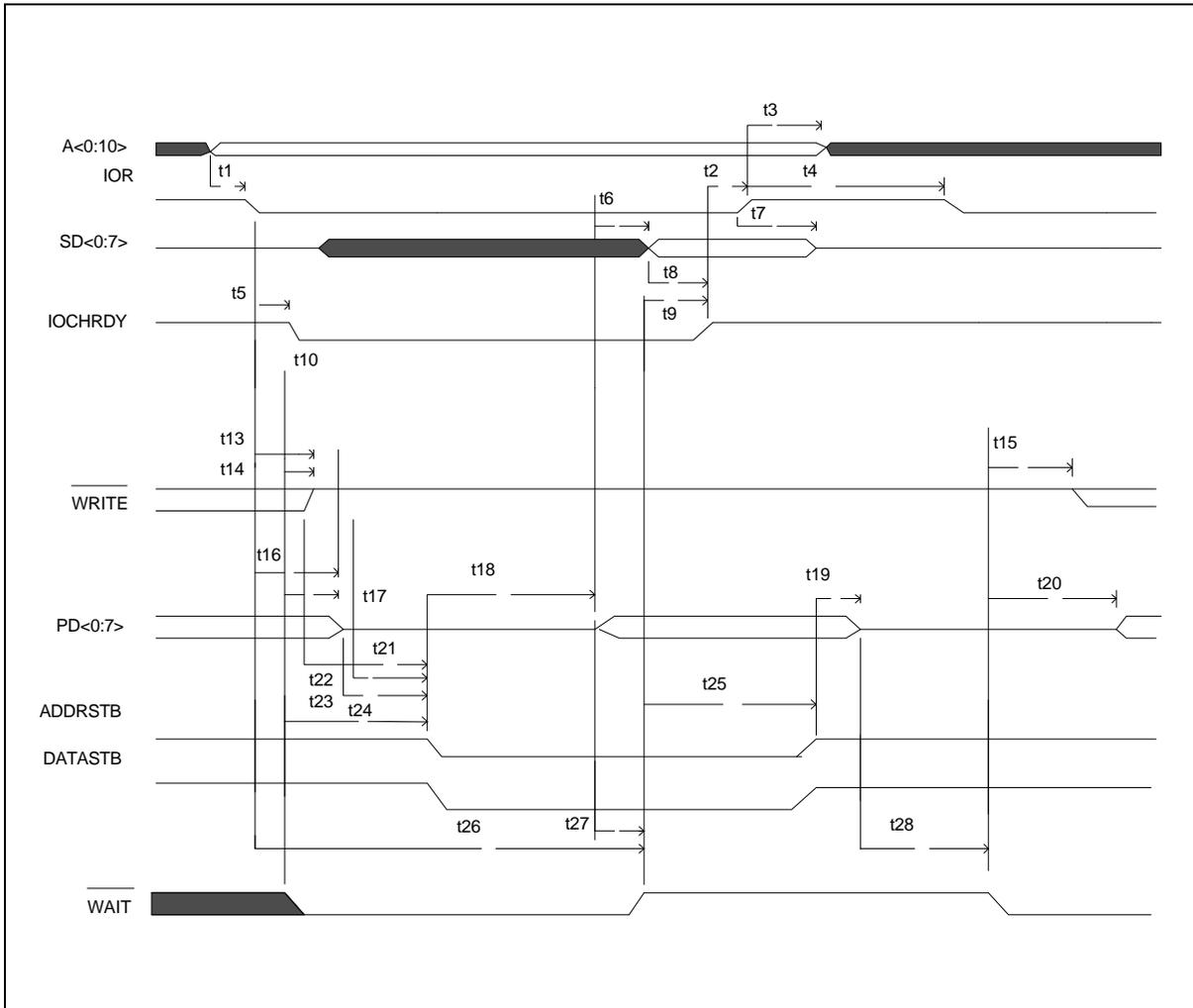
**13.3.3 EPP Data or Address Write Cycle (EPP Version 1.9)**
