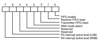
Bit 6, 7: These two bits are used to set the active level for the receiver FIFO interrupt. For example, if the interrupt active level is set as 4 bytes, once there are more than 4 data characters in the receiver FIFO, the interrupt will be activated to notify the CPU to read the data from the FIFO.
