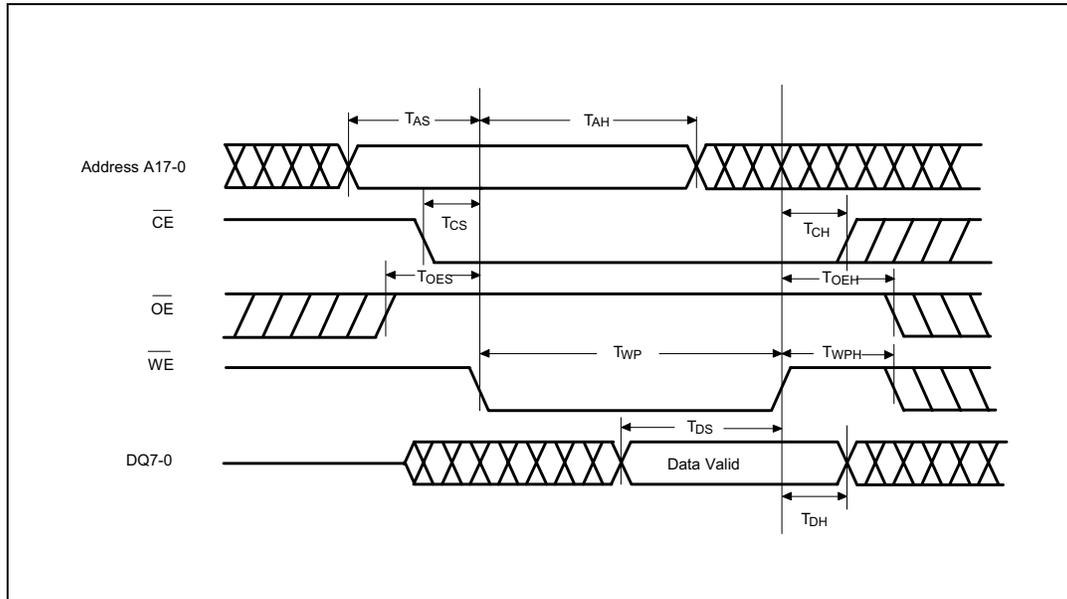
**$\overline{\text{CE}}$  Controlled Command Write Cycle Timing Diagram**
