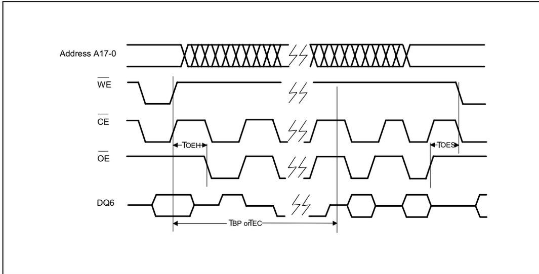
**Boot Block Lockout Enable Timing Diagram**
