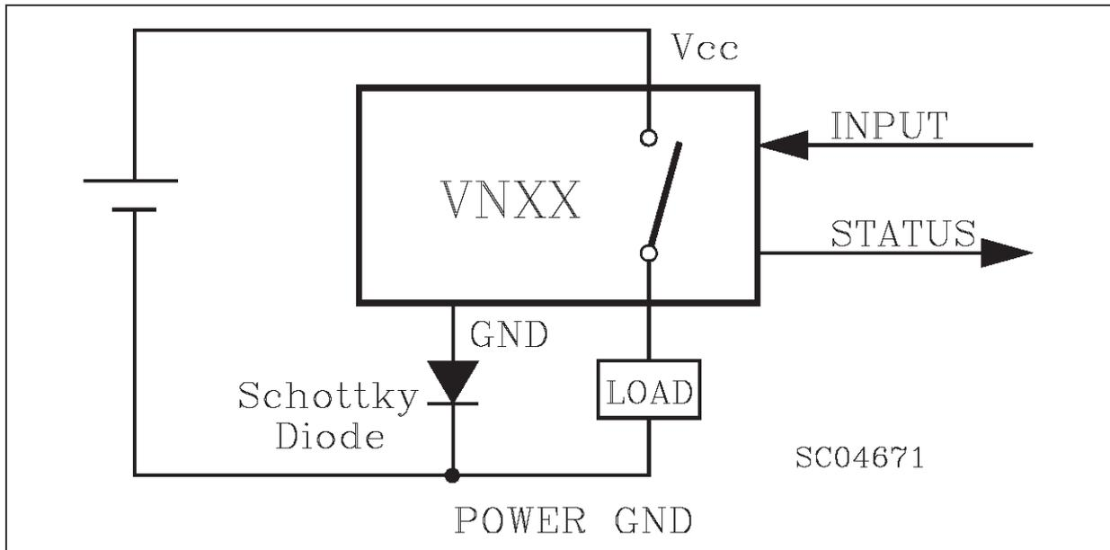
**Figure 4:** Typical Application Circuit With Separate Signal Ground
