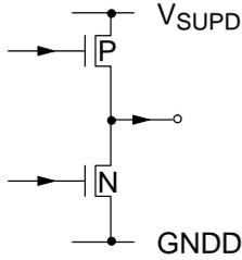
**Fig. 4-13:** Output pins FSY, MSY, CSY, INTLC, PORT[6:0]
