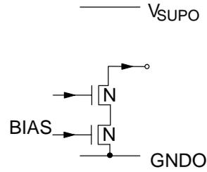
**Fig. 4-17:** Analog output pins ROUT, GOUT, BOUT, SVMOUT
