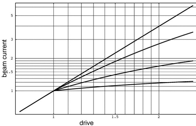
**Fig. 2–24:** Beam current limiter characteristics: beam current output vs. drive
