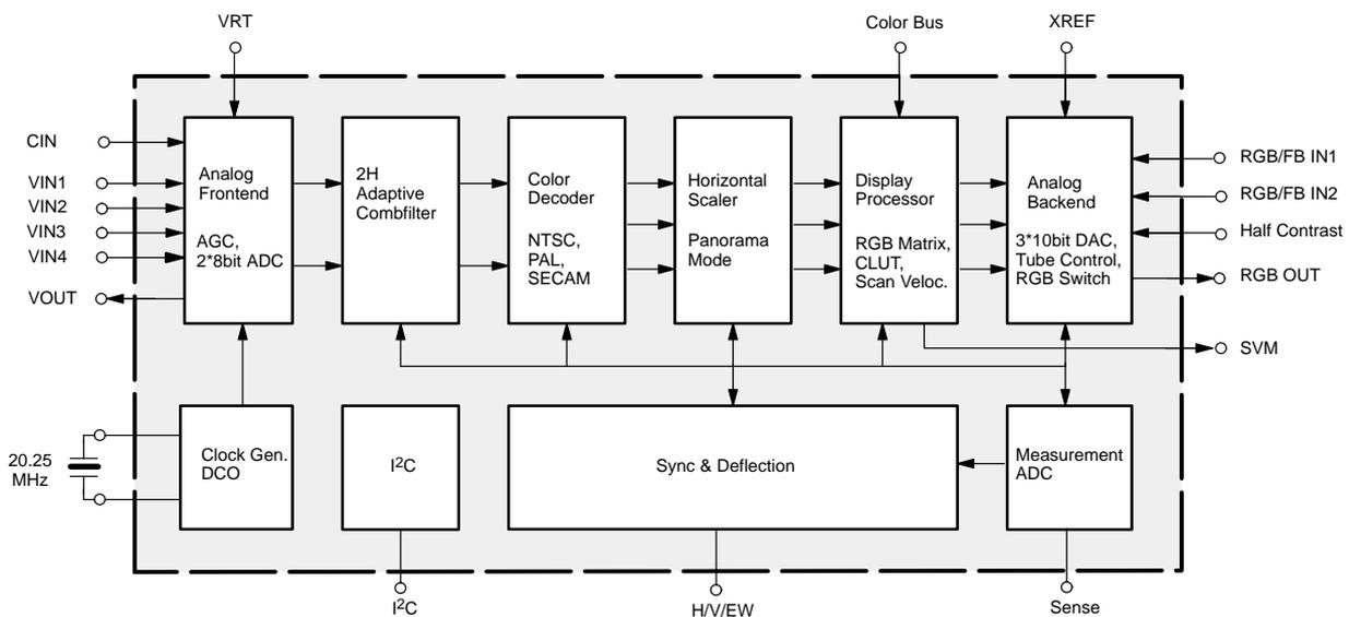
Fig. 1–2: Block diagram of the VDP 3120B
