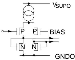
**Fig. 4-15:** Input pins FBLIN1/2, RIN1/2, BIN1/2, GIN1/2, SENSE
