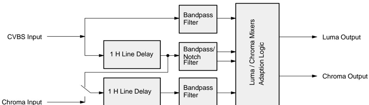
**Fig. 2–3:** Block diagram of the adaptive comb filter
