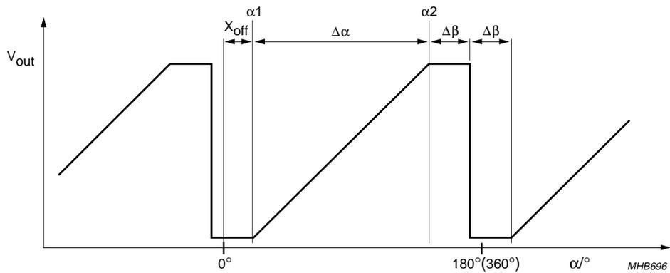
When using MR sensors (KMZ41), the signal period is 0° to 180° as the signals are proportional to  $\sin 2\alpha$  and  $\cos 2\alpha$ .
