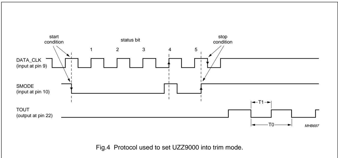
Fig.4 Protocol used to set UZZ9000 into trim mode.
