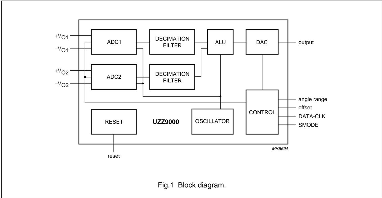
Fig.1 Block diagram.
