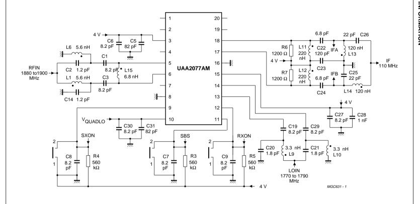
Figure 5 illustrates the electrical diagram of the UAA2077AM Philips demonstration board for DECT applications. All matching is to 50  $\Omega$  for measurement purposes. Different values will be used in a real application.
