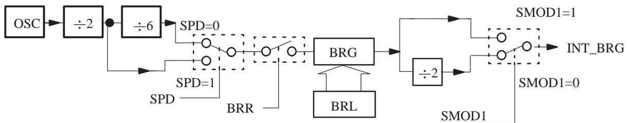
**Figure 4.7. Internal Baud Rate Generator in modes 1 and 3**
