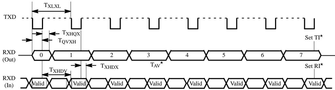
\* TI and RI are set during S1P1 of the peripheral cycle following the shift of the eight bit.
