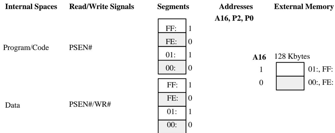
**Figure 1.6. Internal/external memory segments (RD1:0 = 01)**
