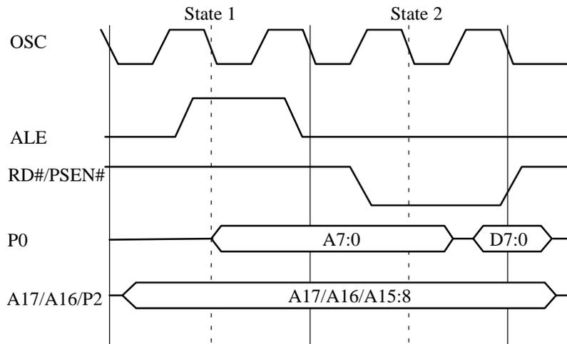
**Figure 1.2. External bus cycle: code fetch, non-page mode**
