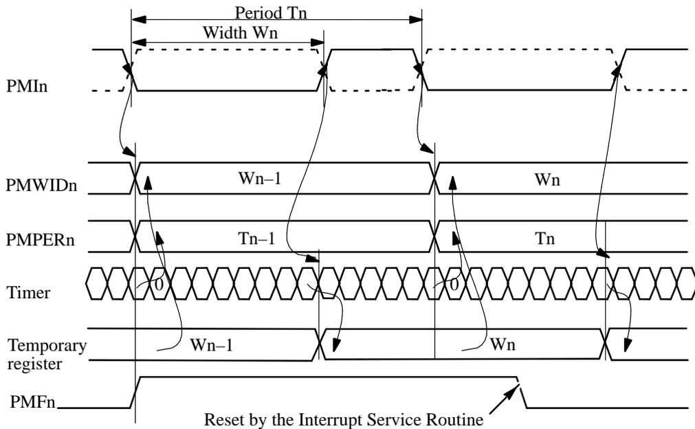
**Figure 5.3. PMU measurement**
