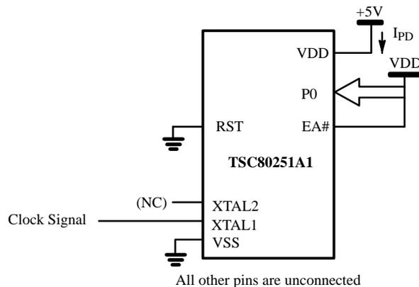
**Figure 1.1. I<sub>PD</sub> Test Condition, Power-Down mode**
