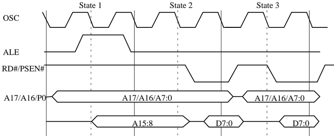
**Figure 1.3. External bus cycle: code fetch, page mode**
