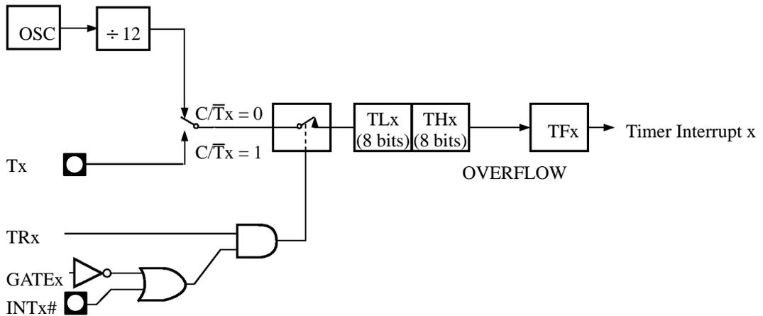
**Figure 3.2. Timer/Counter x (x = 0 or 1) in mode 1**
