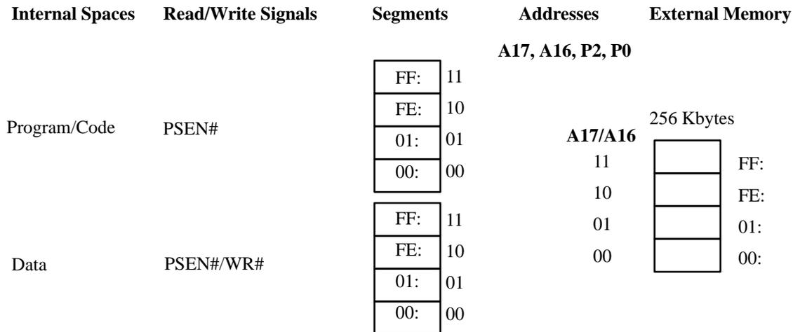
**Figure 1.5. Internal/external memory segments (RD1:0 = 00)**
