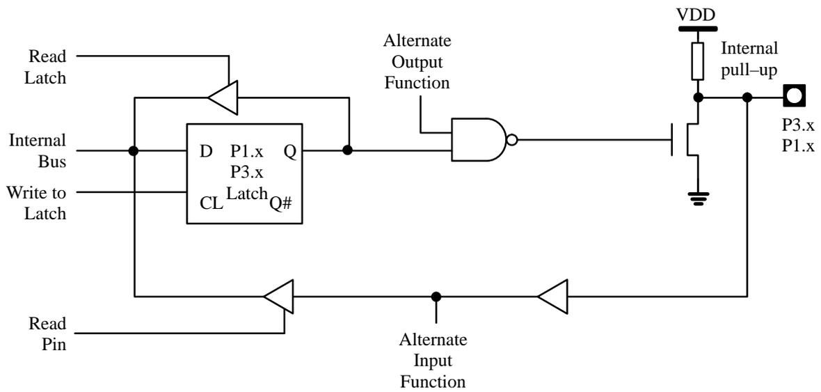
**Figure 2.1. Port 1 and Port 3 structure**
