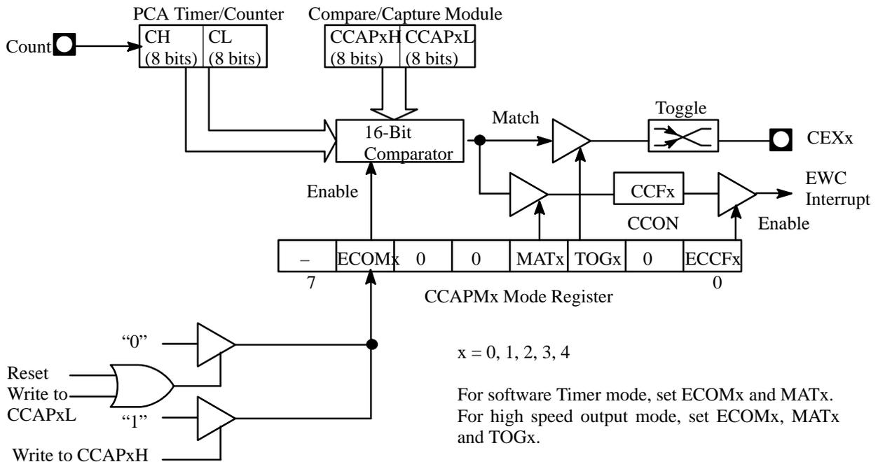
**Figure 6.3. PCA Software Timer and High-Speed Output Modes**
