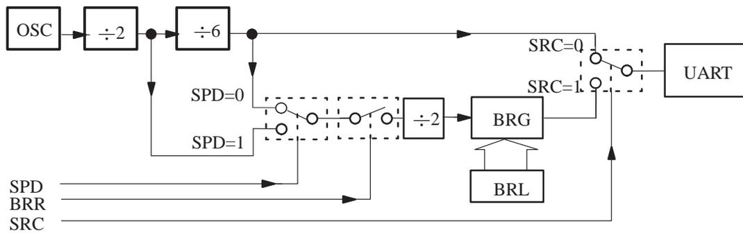
**Figure 4.5. Clock transmission sources in mode 0**
