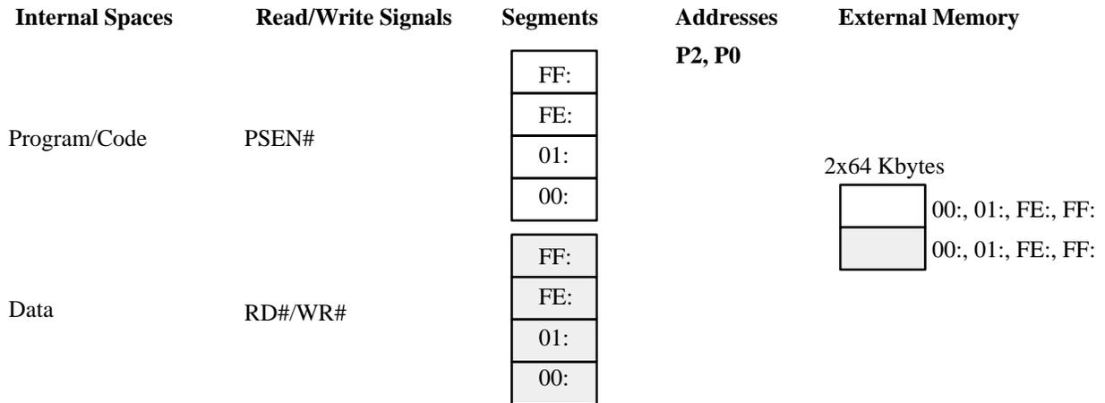
**Figure 1.8. Internal/external memory segments (RD1:0 = 11)**
