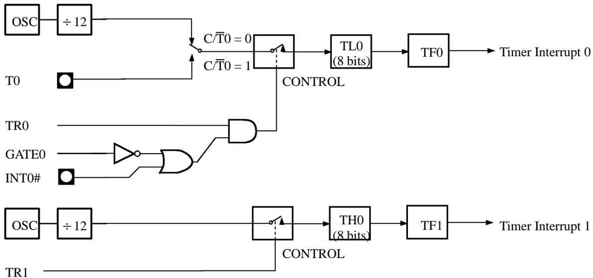
**Figure 3.4. Timer/Counter in mode 3 : Two 8-bit Counters**
