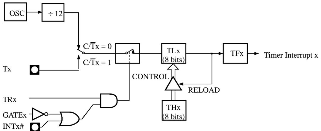
**Figure 3.3. Timer/Counter x (x = 0 or 1) in mode 2**
