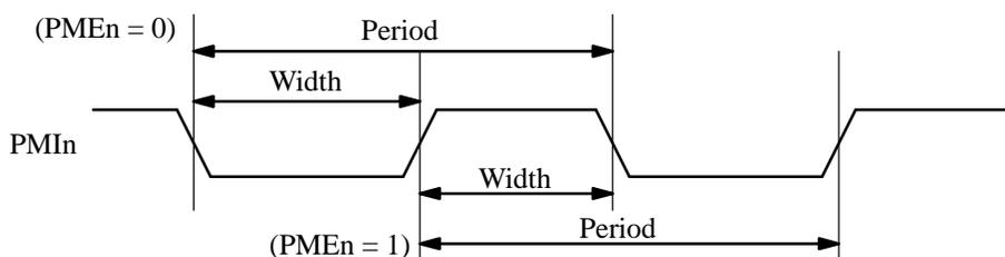
**Figure 5.4. Pulse measurement polarity**
