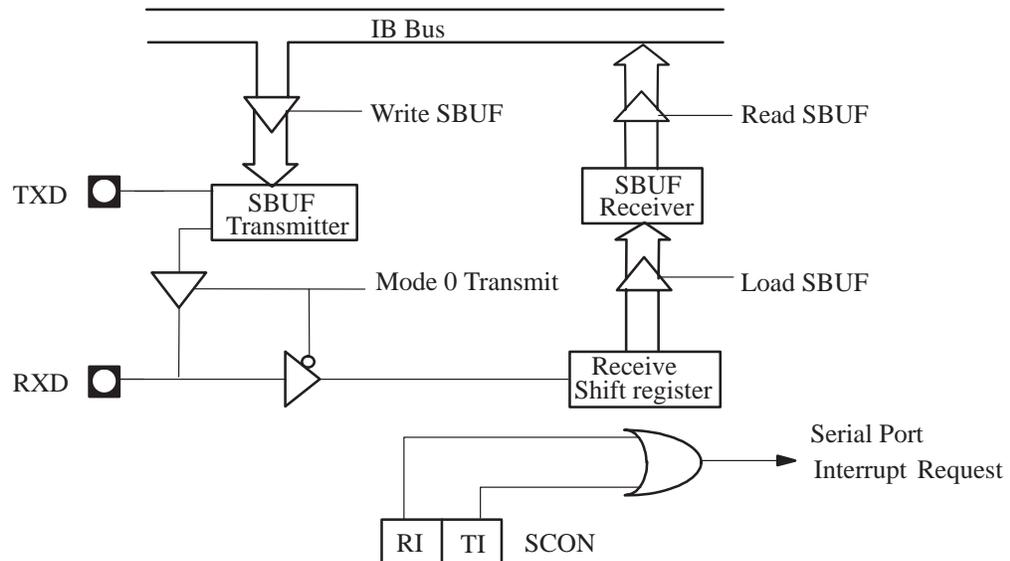
**Figure 4.1. Serial Port block diagram**
