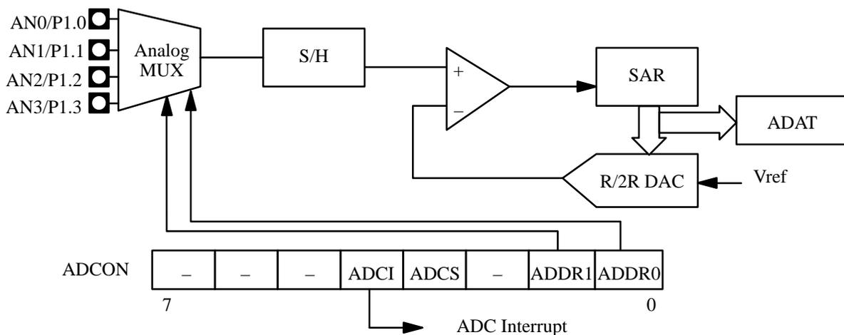
**Figure 7.1. Analog Digital Converter structure**
