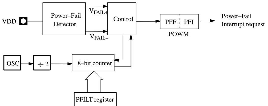
**Figure 8.4. Block diagram of the digital filter**
