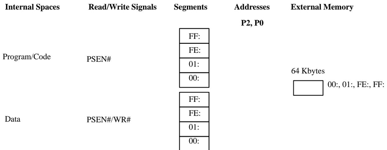
**Figure 1.7. Internal/external memory segments (RD1:0 = 10)**
