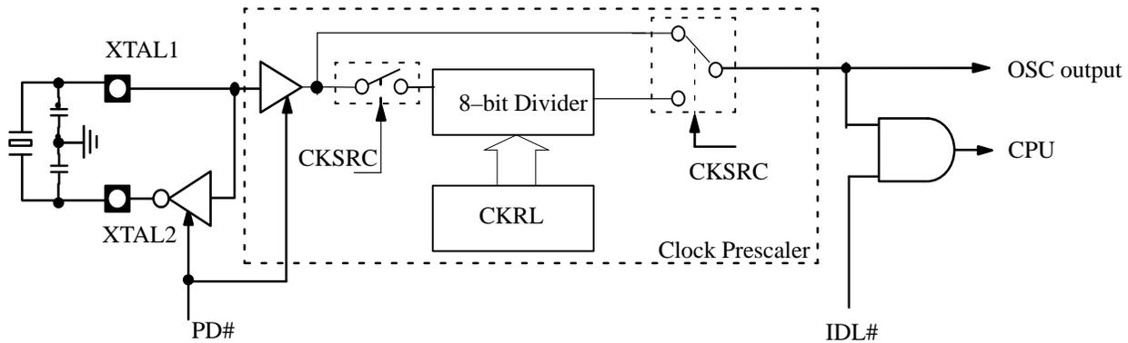
**Figure 8.6. Block diagram of the on-chip oscillator**
