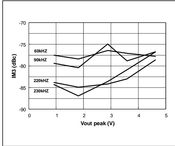
**3rd Order Intermodulation (2 tones : 180kHz and 280kHz)**
