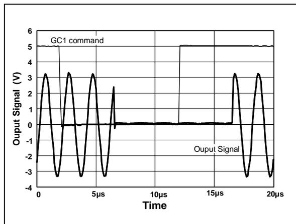
measurement conditions:  $V_{cc}=\pm 6V$ ,  $R_{load}=500\Omega$ ,  $T_{amb}=25^{\circ}C$
