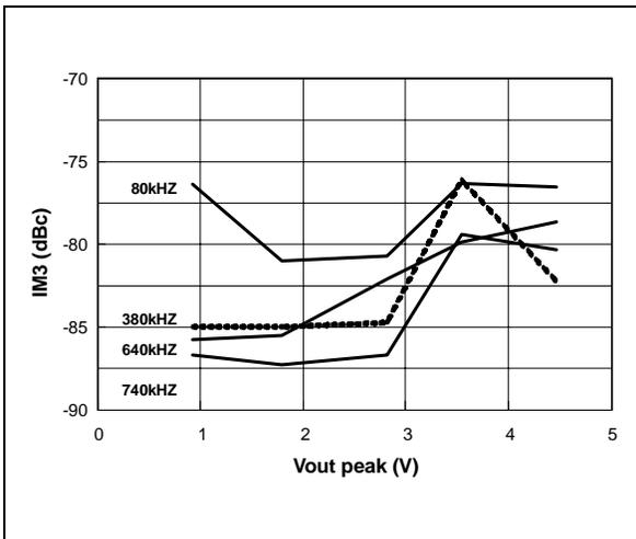
measurement conditions: Vcc=±6V, Rload=500Ω, Tamb=25°C
