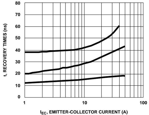
FIGURE 12. TYPICAL  $t_{RR}$ ,  $t_A$ ,  $t_B$  vs FORWARD CURRENT
