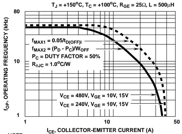
NOTE: PD = ALLOWABLE DISSIPATION PC = CONDUCTION DISSIPATION
