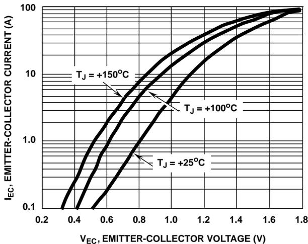
FIGURE 11. FORWARD VOLTAGE vs FORWARD CURRENT CHARACTERISTIC
