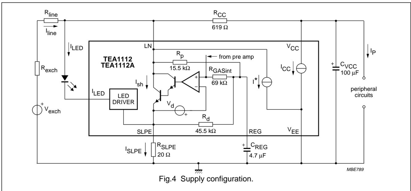
Fig.4 Supply configuration.
