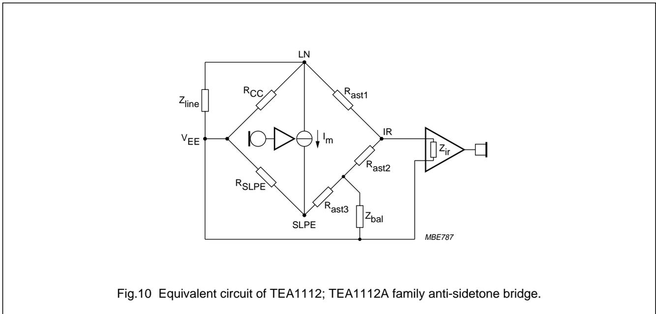
Fig.10 Equivalent circuit of TEA1112; TEA1112A family anti-sidetone bridge.
