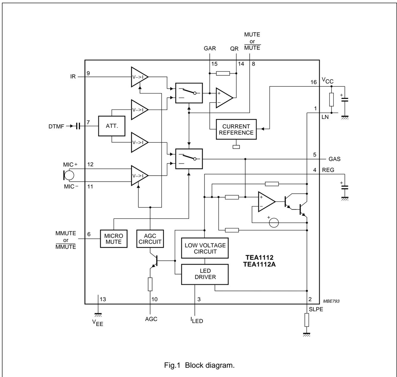
Fig.1 Block diagram.
