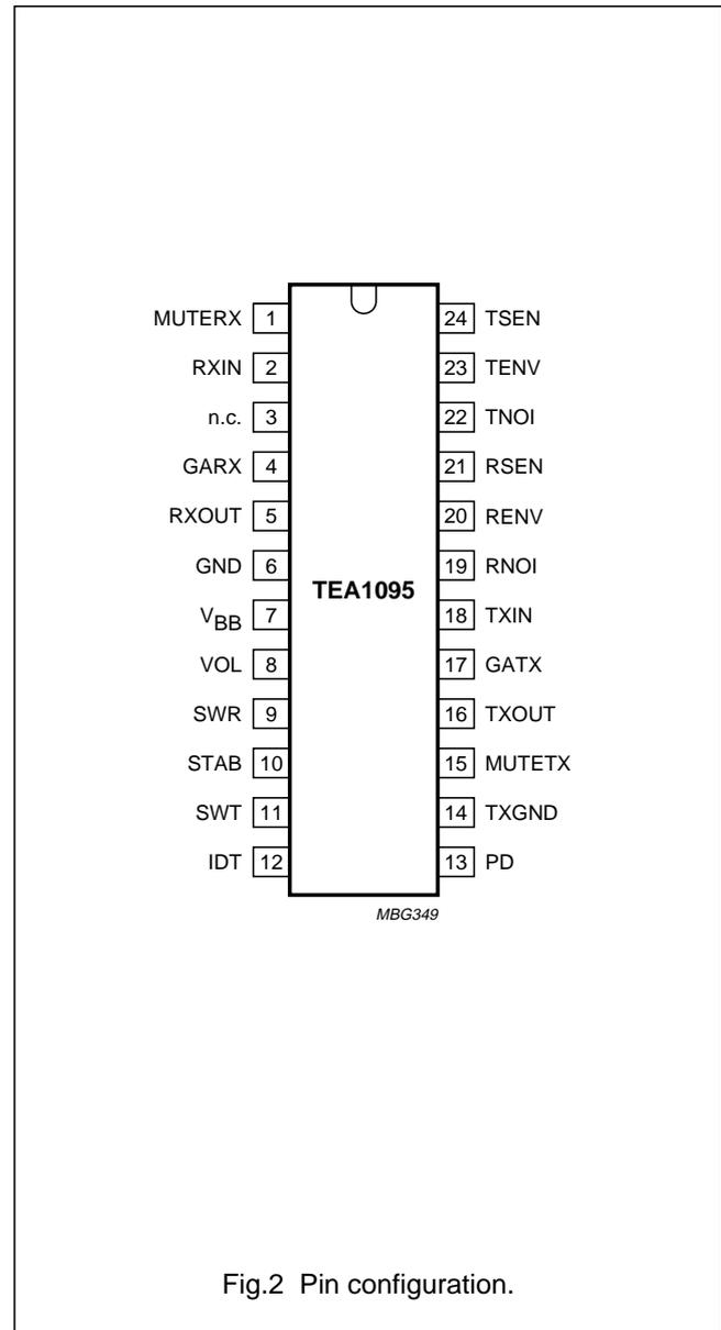
Fig.2 Pin configuration.
