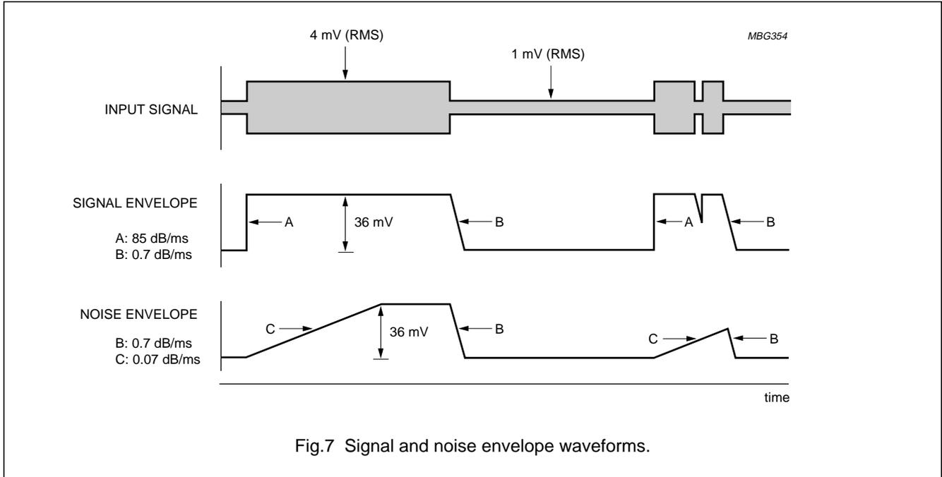
Fig.7 Signal and noise envelope waveforms.
