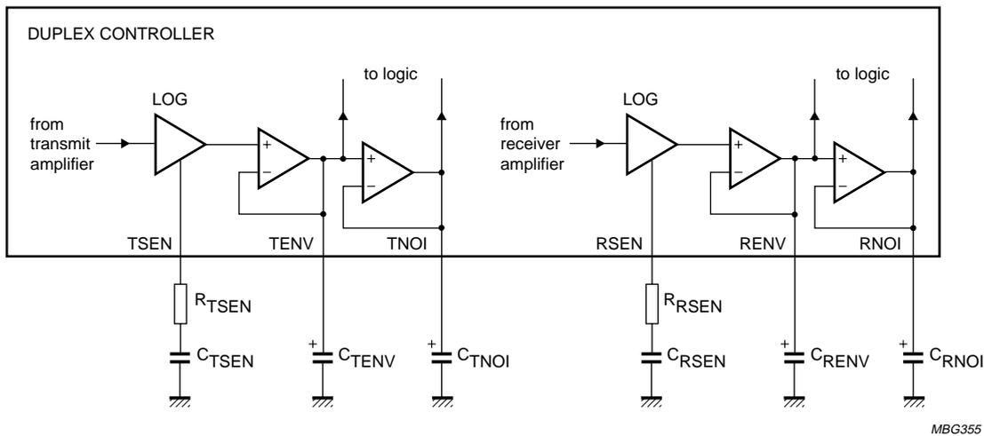
Fig.6 Signal and noise envelope detectors.
