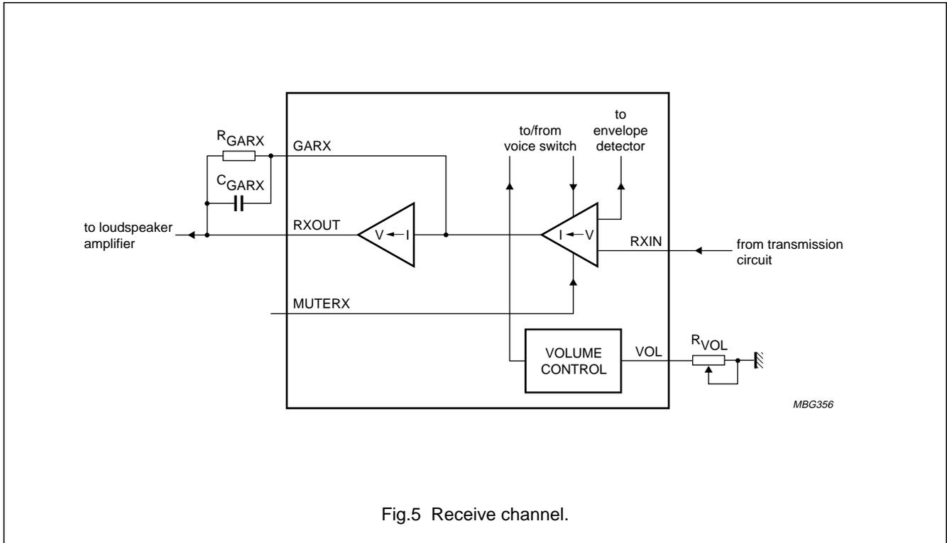
Fig.5 Receive channel.
