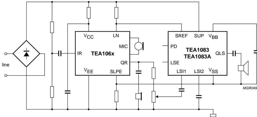
Fig.5 Interconnection with a transmission IC of the TEA106X family.
