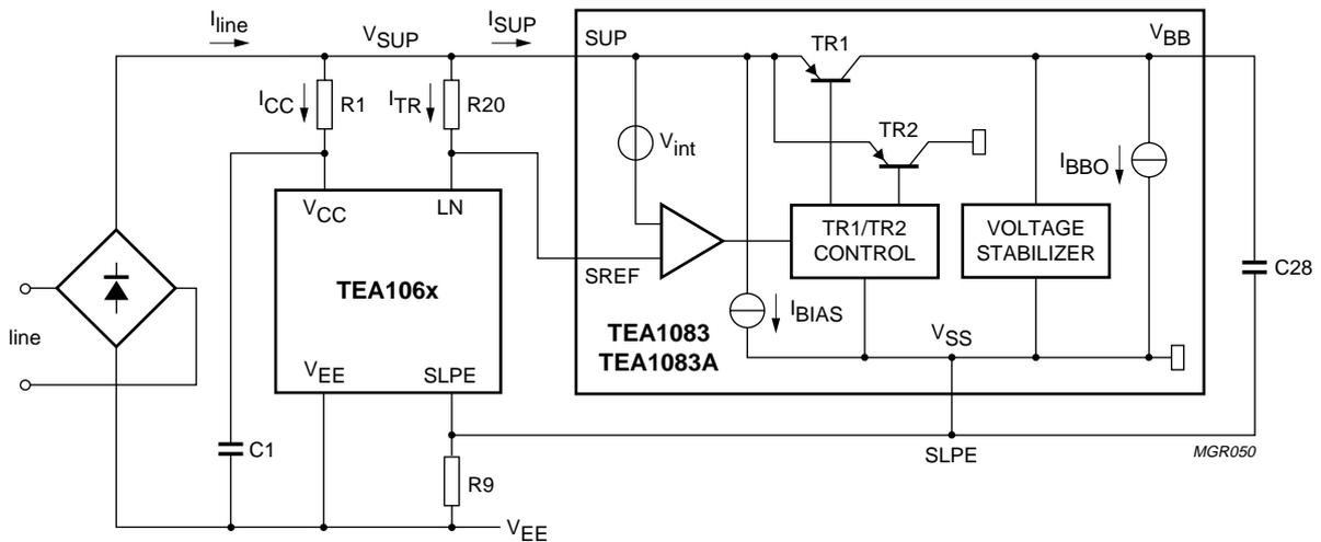
Fig.6 Supply arrangement.
