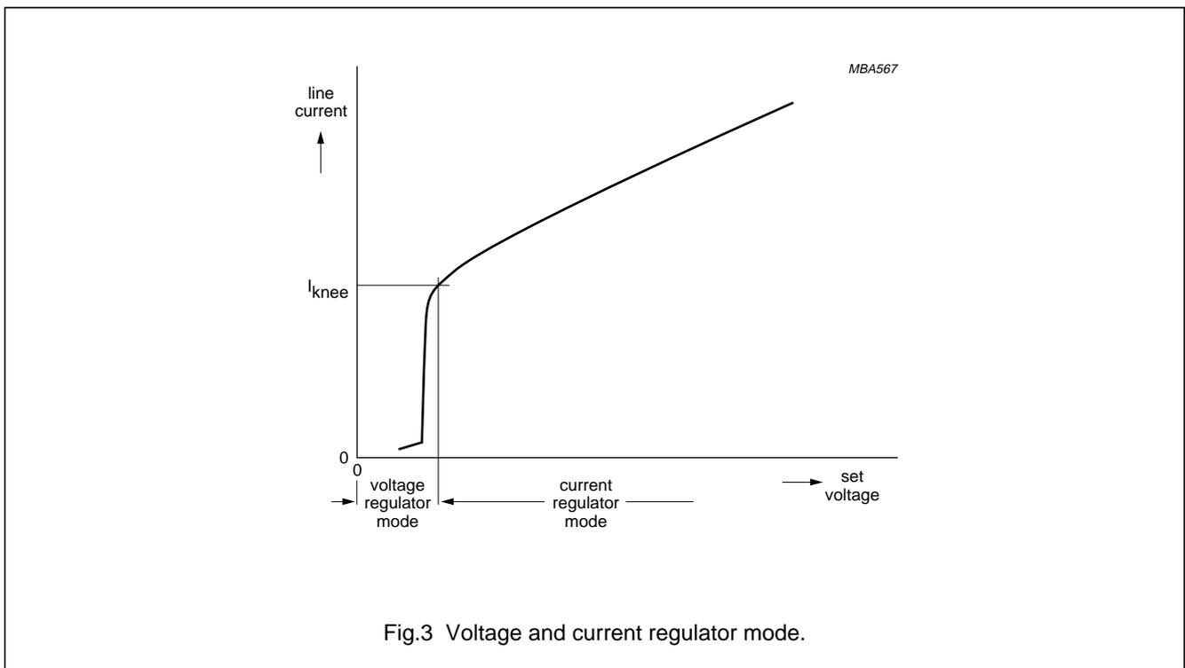
Fig.3 Voltage and current regulator mode.
