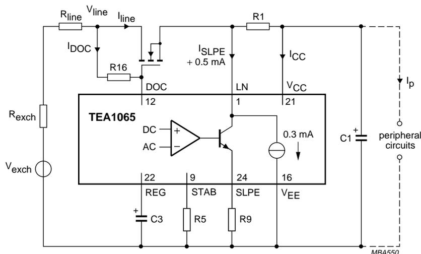
Fig.4 Supply arrangement.
