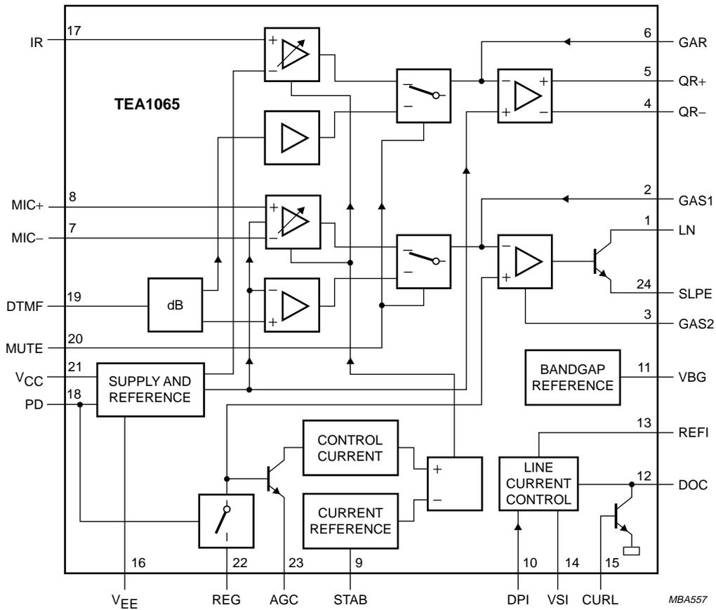
Fig.1 Block diagram.
