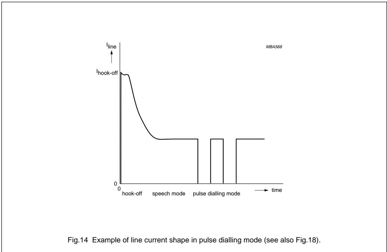
Fig.14 Example of line current shape in pulse dialling mode (see also Fig.18).
