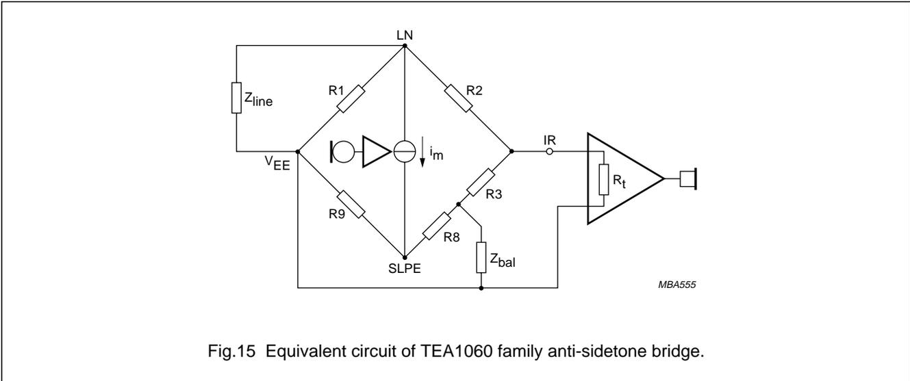
Fig.15 Equivalent circuit of TEA1060 family anti-sidetone bridge.
