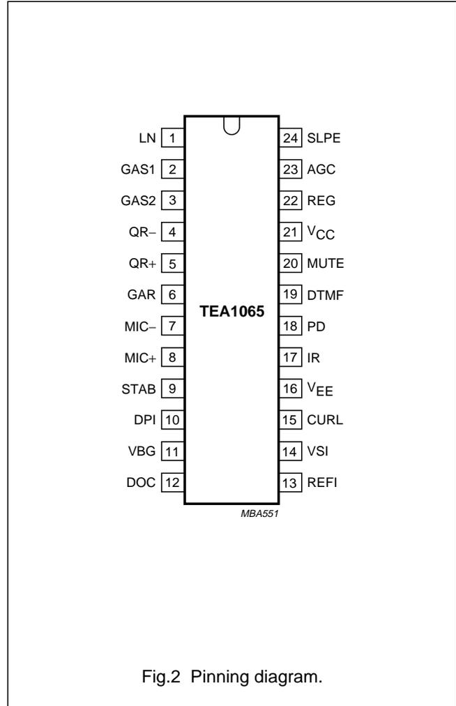
Fig.2 Pinning diagram.
