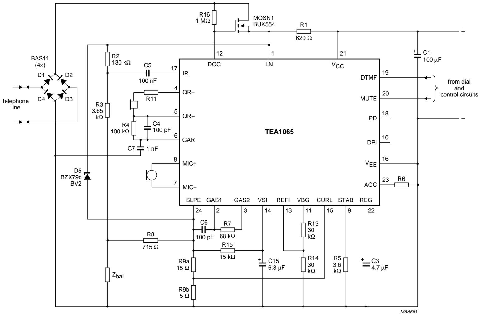
Fig.18 Typical application of the TEA1065, with a piezoelectric earpiece and DTMF dialling.
