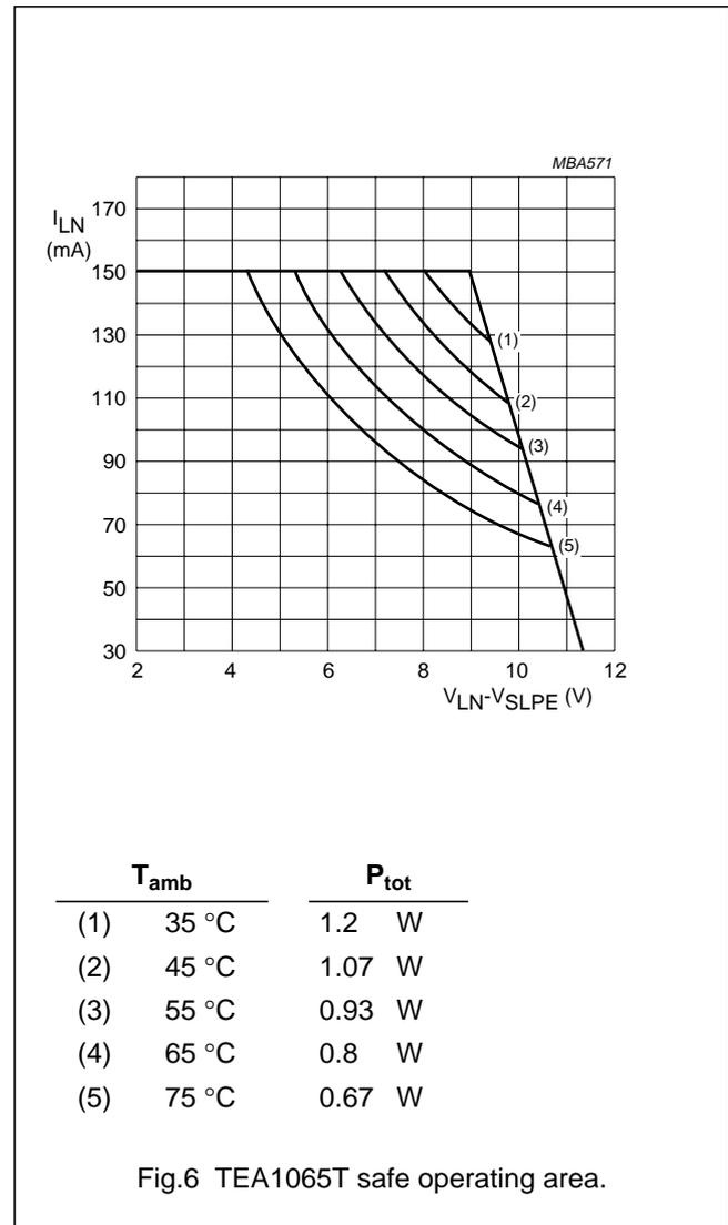
Versatile telephone transmission circuit with dialler interface
