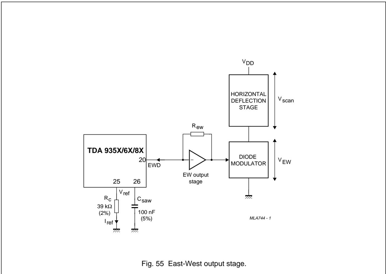
Fig. 55 East-West output stage.
