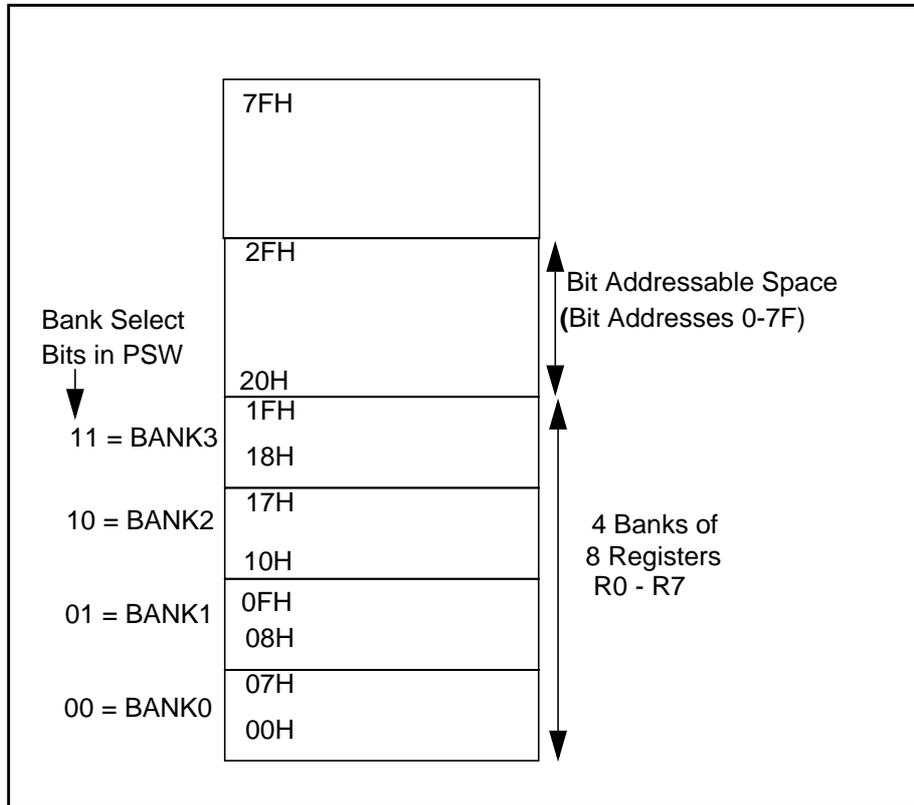
Figure 10 Lower 128 Bytes of Internal RAM
