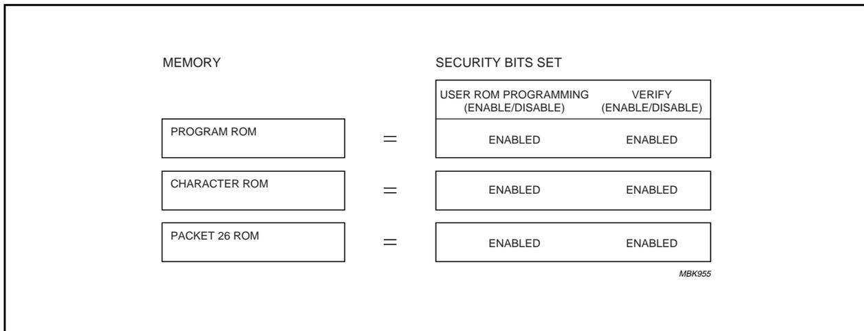
**Figure 8 Security bits for production blank devices**
