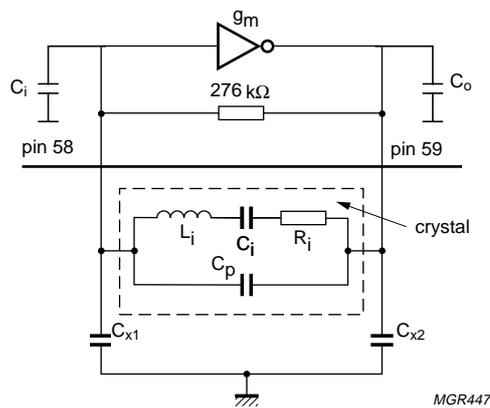
$$f_{osc} = \frac{1}{2\pi \sqrt{L_i \times \frac{C_i \times C_{tot}}{C_i + C_{tot}}}}$$
