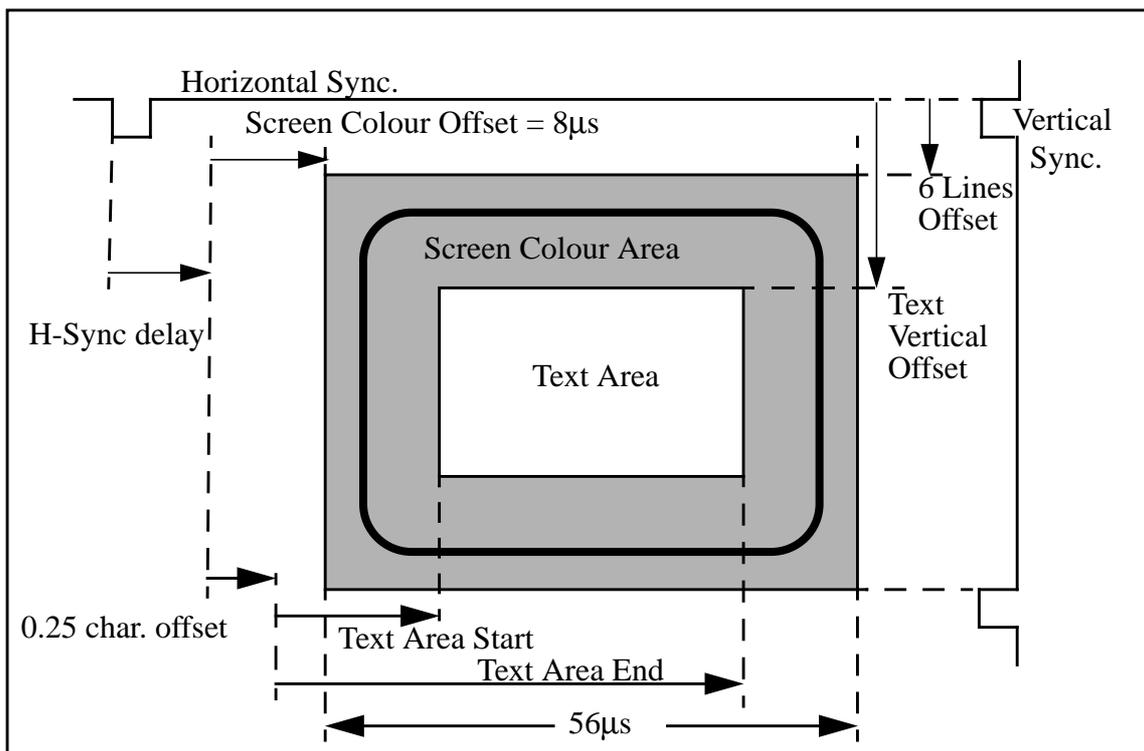
**Figure 36 Display Area Positioning**
