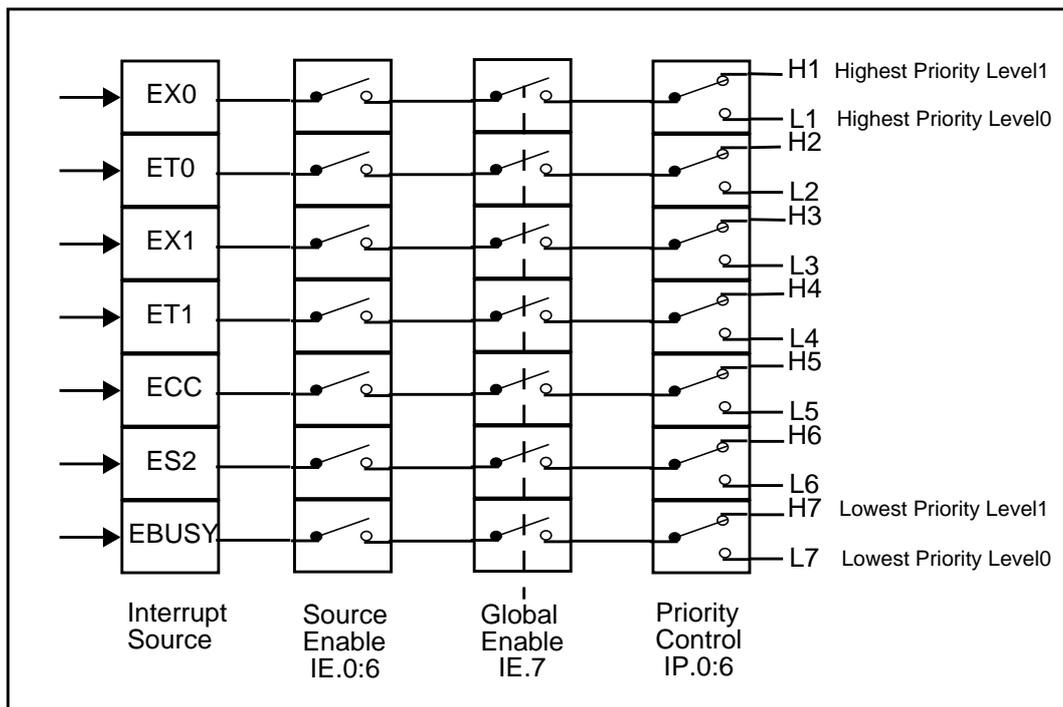
**Figure 13 Interrupt Structure**
