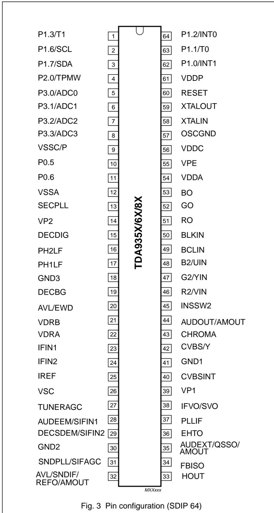
TV signal processor-Teletext decoder with embedded  $\mu$ -Controller
