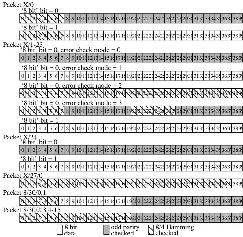
Figure 19 Error Checking
