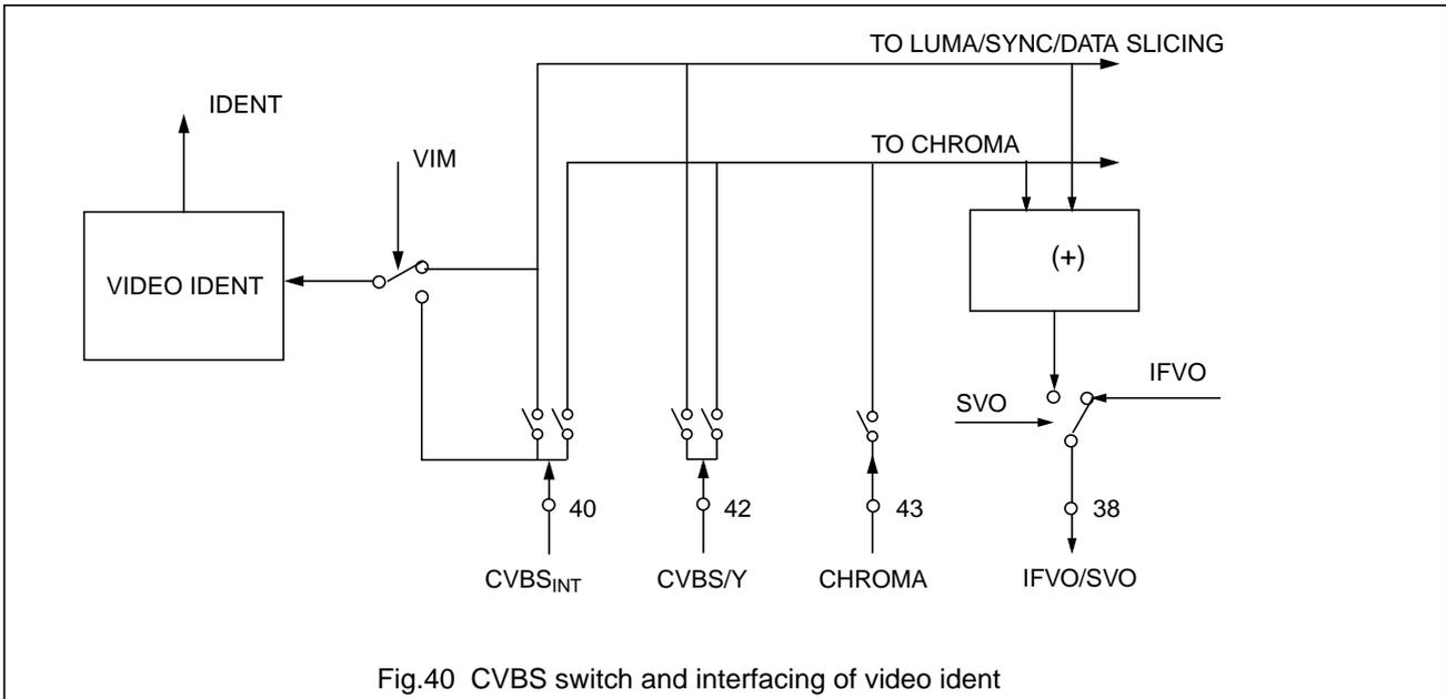
Fig.40 CVBS switch and interfacing of video ident
