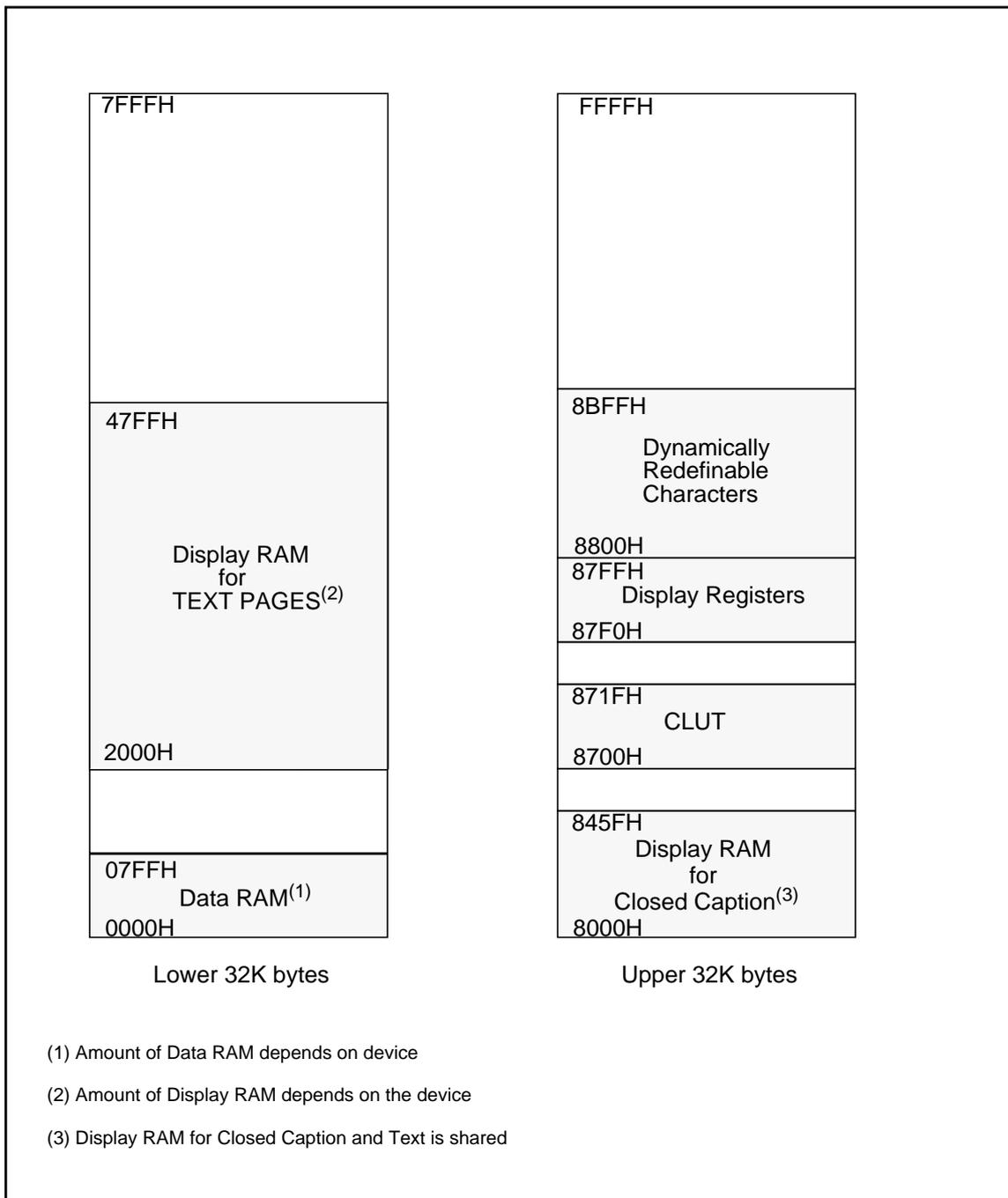
Figure 11 Auxiliary RAM allocation
