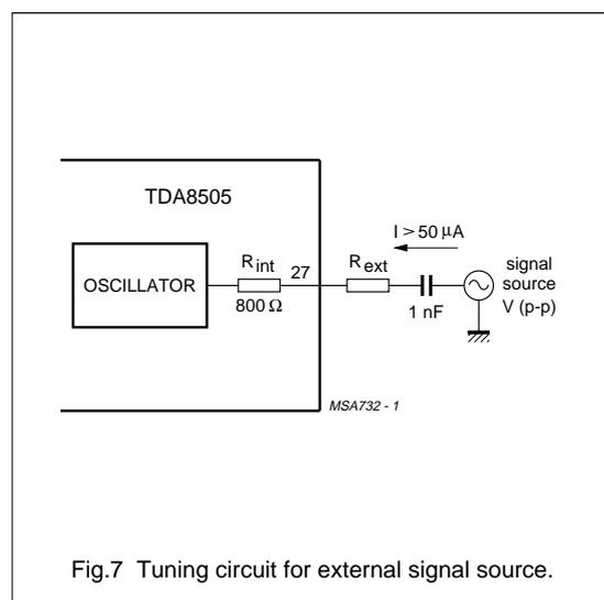
Fig.7 Tuning circuit for external signal source.
