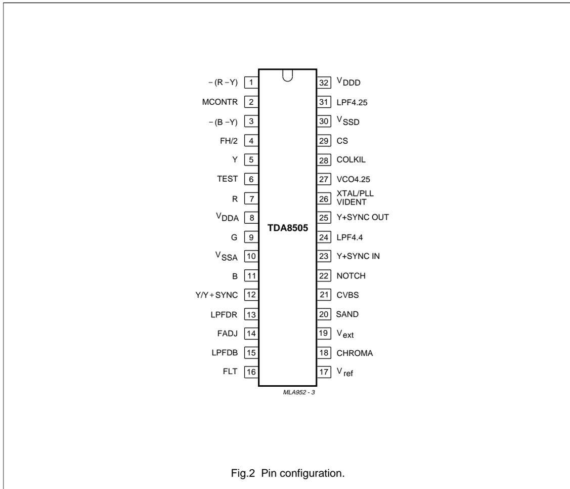
Fig.2 Pin configuration.
