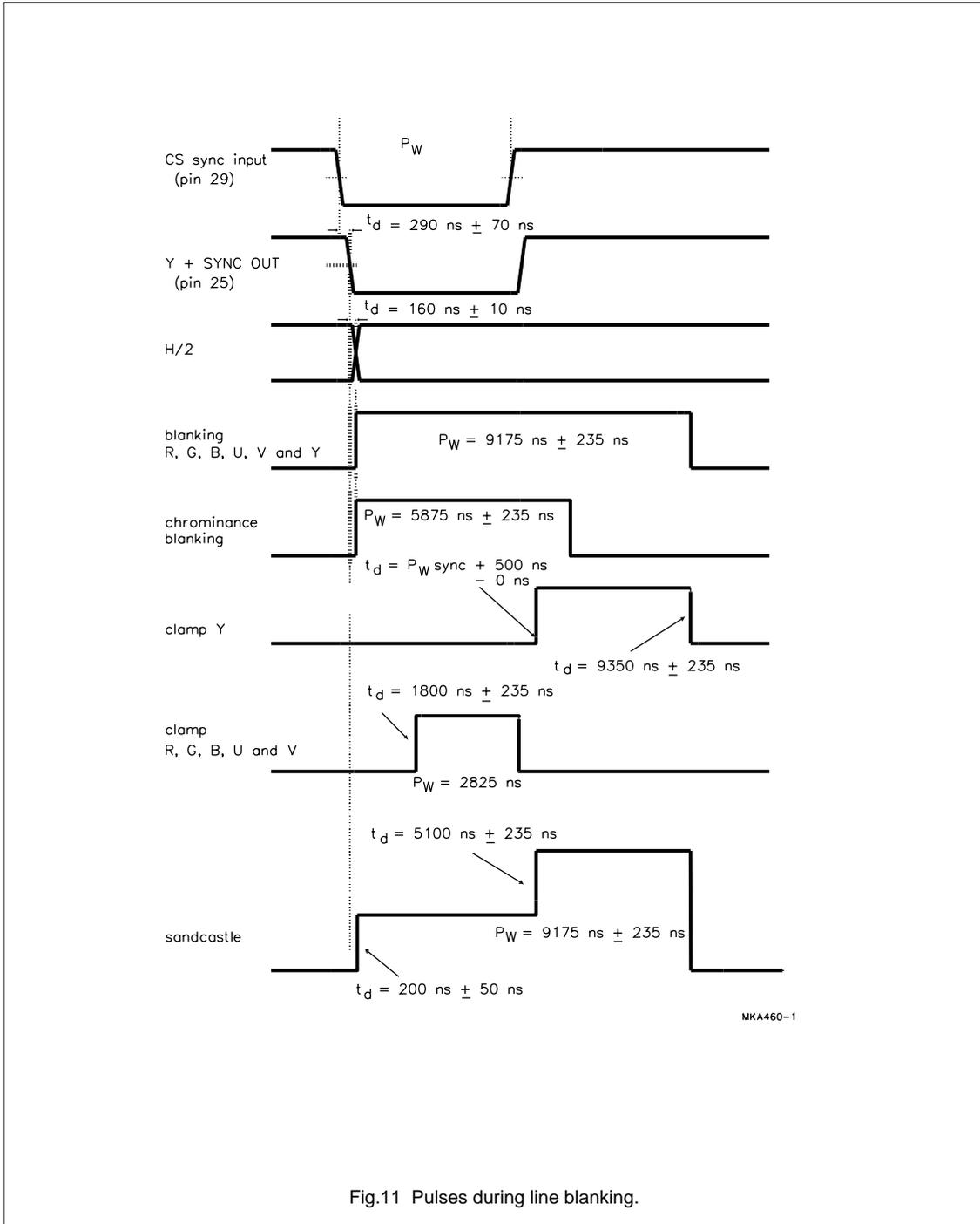
Fig.11 Pulses during line blanking.
