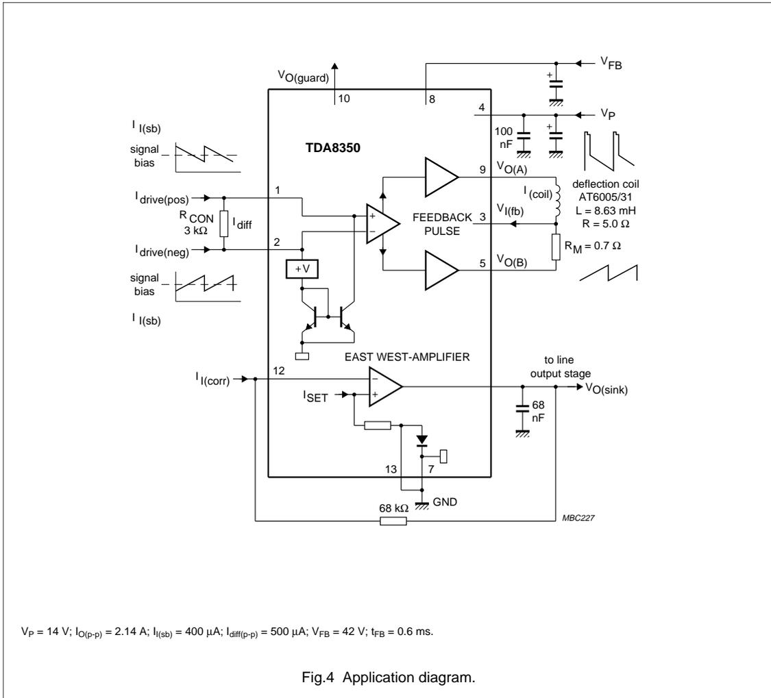
DC-coupled vertical deflection and East-West output circuit
