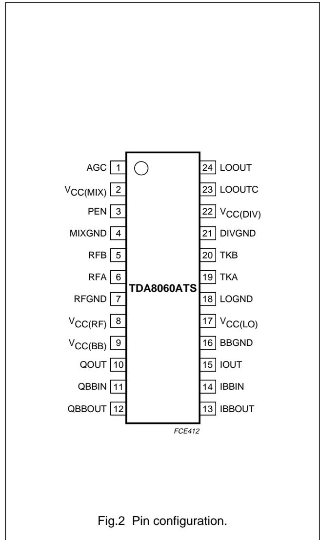
Fig.2 Pin configuration.
