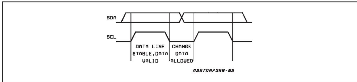
**Figure 4:** Timing Diagram of I<sup>2</sup>C BUS
