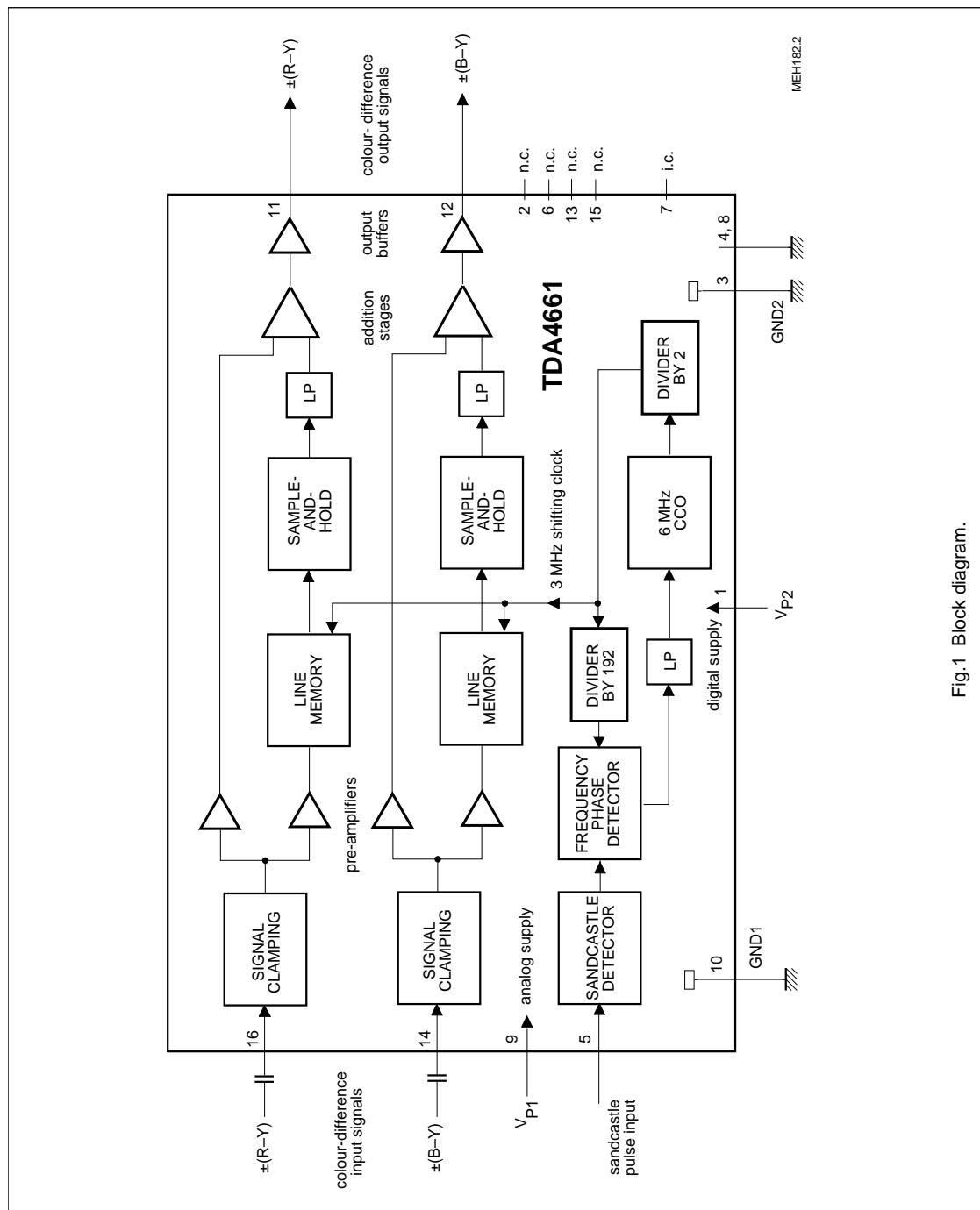
Fig.1 Block diagram.
