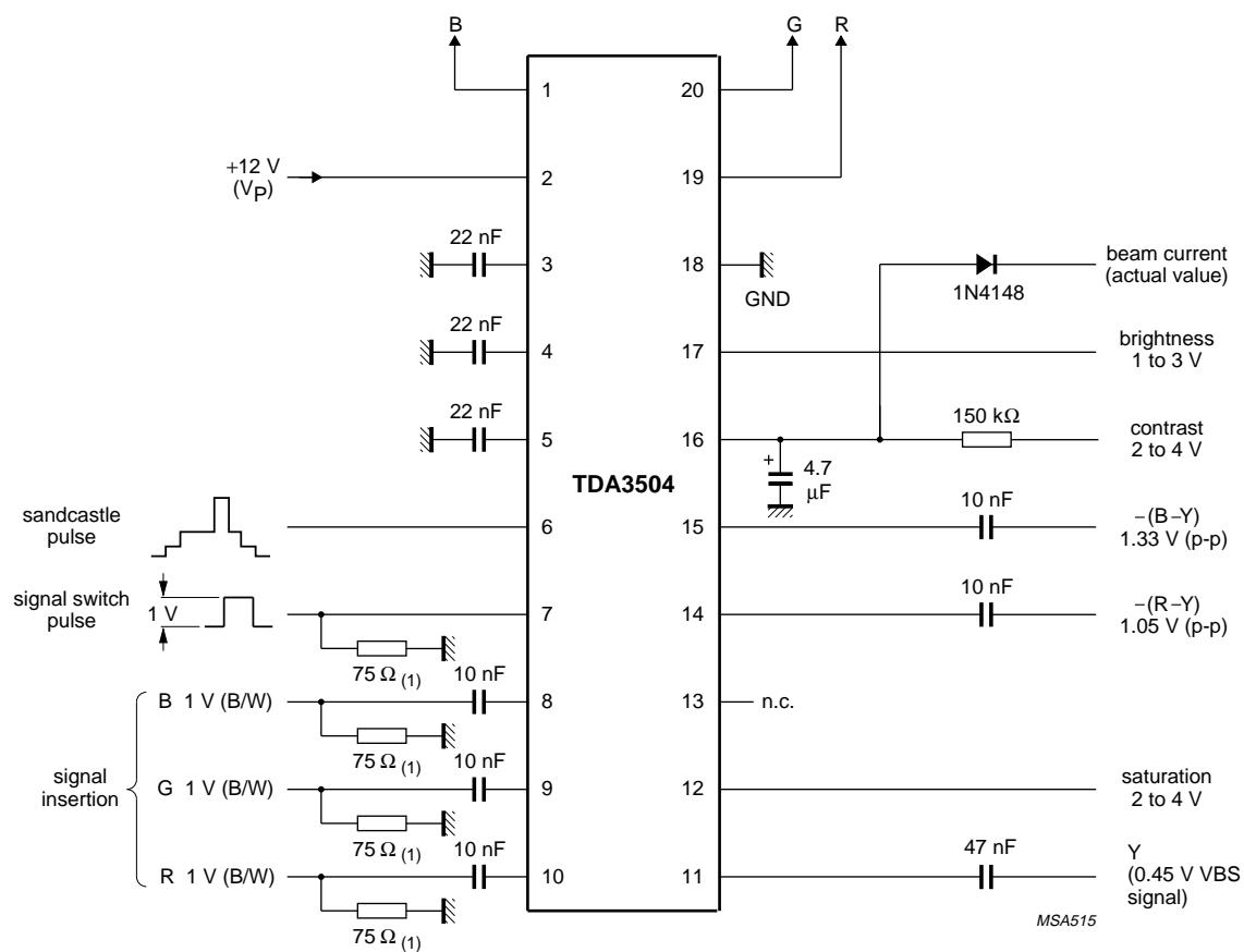
Fig.3 Basic application circuit diagram.
