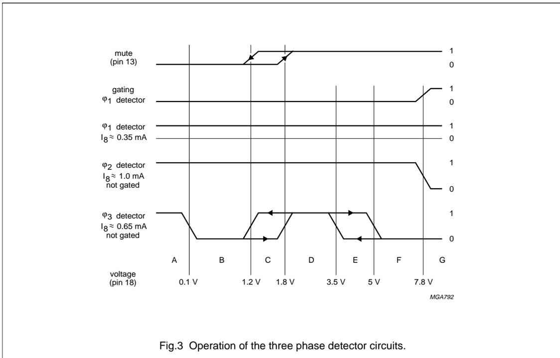
Fig.3 Operation of the three phase detector circuits.
