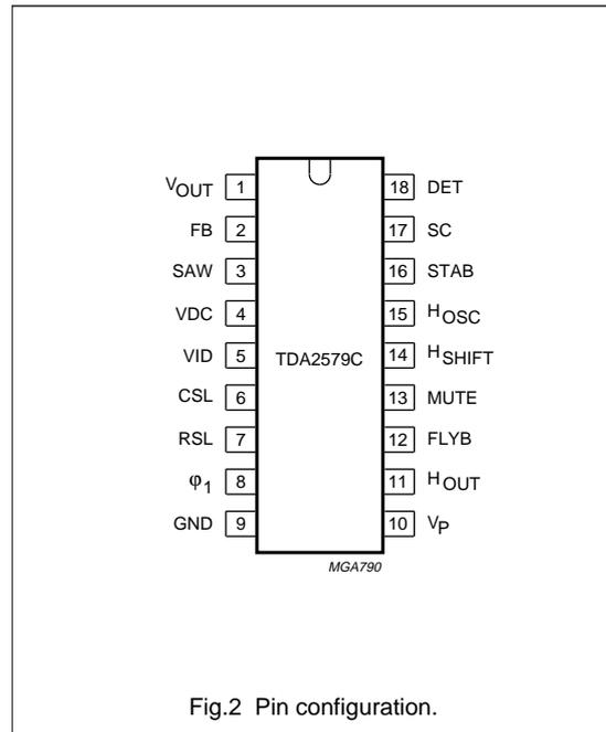
Fig.2 Pin configuration.
