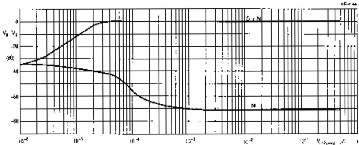
Fig.3 AF output voltage level on pins 8 and 9 as a function of  $V_{i\text{ IF}}$  at  $V_P = 8.5\text{ V}$ ;
