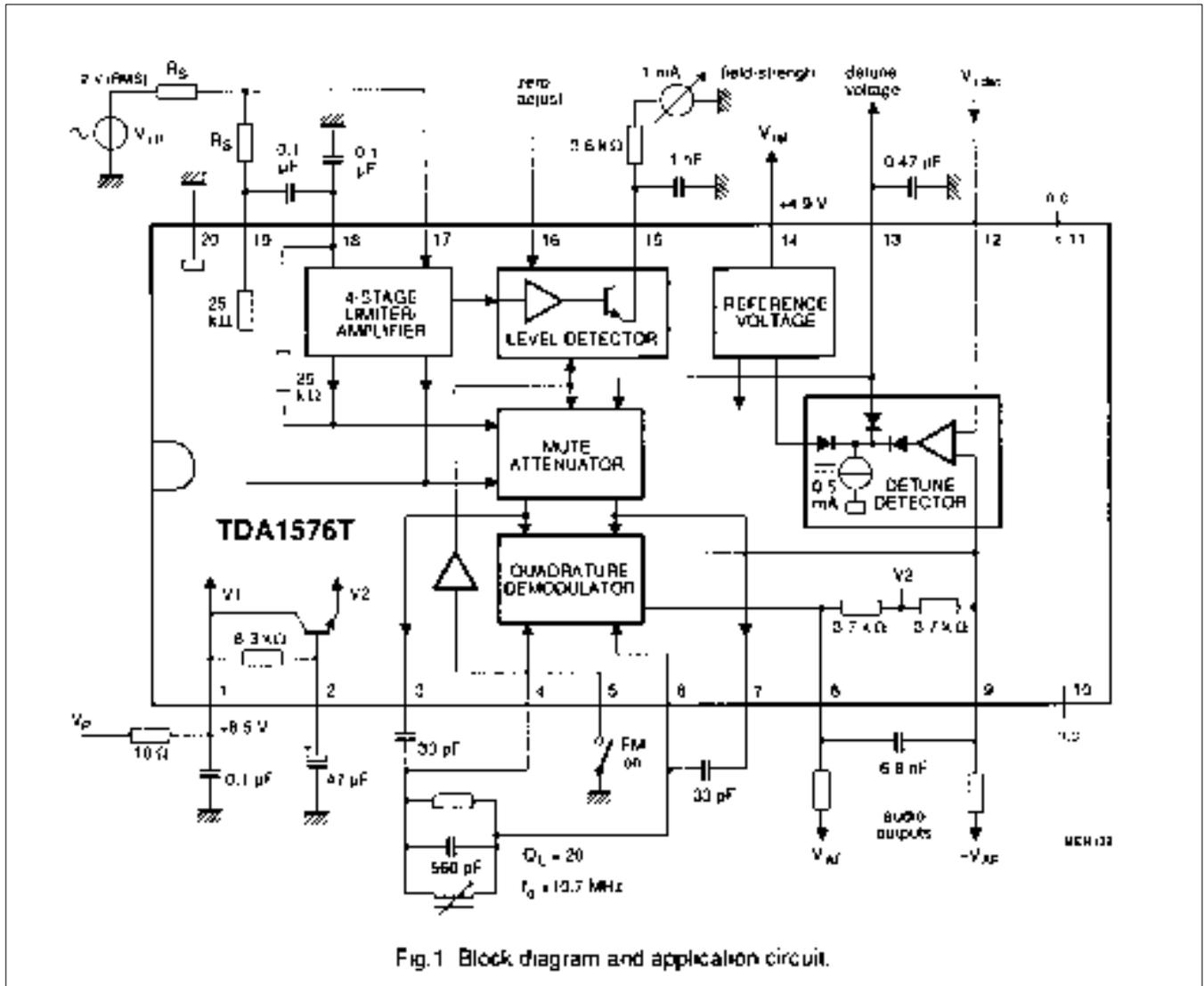
Fig.1 Block diagram and application circuit.
