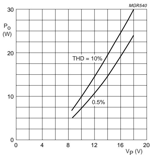
Fig.8 Output power ( $P_o$ ) as a function of supply voltage ( $V_P$ ) for BTL application at  $R_L = 4 \Omega$ ;  $f = 1$  kHz.
