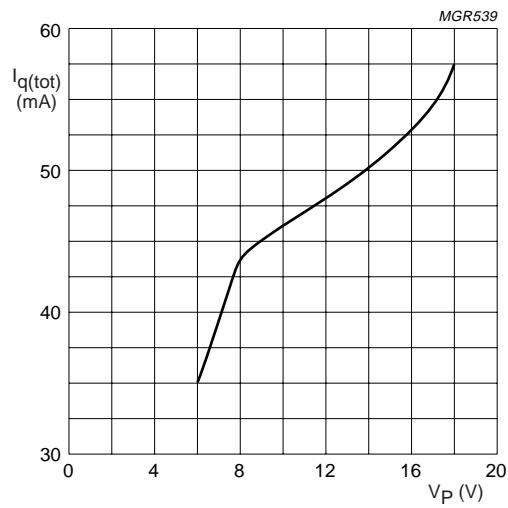
Fig.7 Total quiescent current ( $I_{q(\text{tot})}$ ) as a function of supply voltage ( $V_P$ ).
