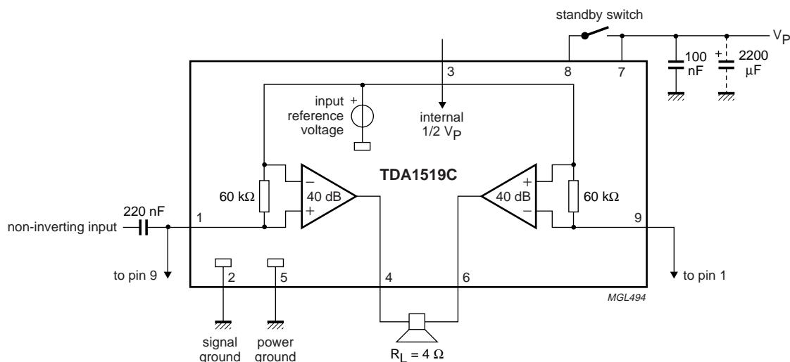
Fig.6 BTL application diagram (SOT131-2 and SOT354-1).
