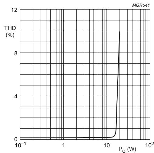
Fig.9 Total harmonic distortion (THD) as a function of output power ( $P_o$ ) for BTL application at  $R_L = 4 \Omega$ ;  $f = 1$  kHz.
