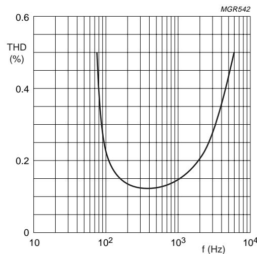
Fig.10 Total harmonic distortion (THD) as a function of operating frequency ( $f$ ) for BTL application at  $R_L = 4 \Omega$ ;  $P_o = 1$  W.
