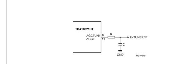
R and C are chosen to verify  $\frac{SR}{1024} < f_c < \frac{XIN}{16}$  with R = 1.5 k $\Omega$  and C = 1 nF,  $f_c$  = 100 kHz.
