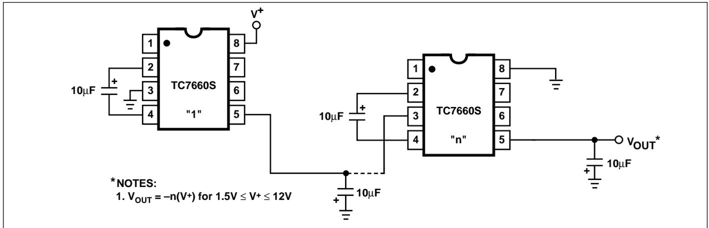
Figure 5. Increased Output Voltage by Cascading Devices
