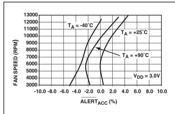
**FIGURE 2-5:** Fan Speed vs.  $\overline{ALERT} ACC$ .
