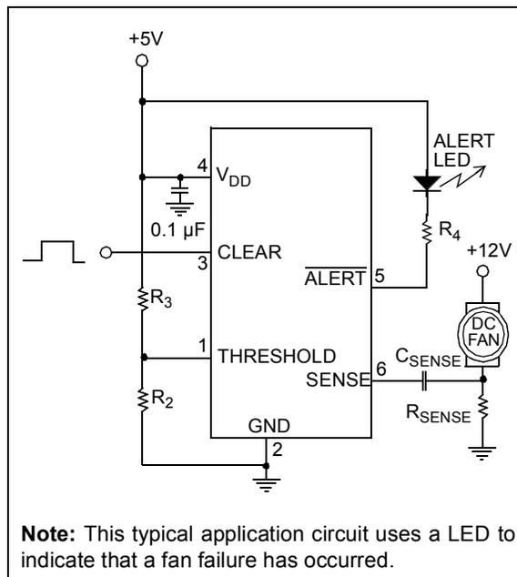
**Note:** This typical application circuit uses a LED to indicate that a fan failure has occurred.
