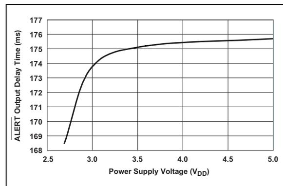
**FIGURE 2-6:**  $\overline{ALERT}$  Output Delay vs. Power Supply Voltage.
