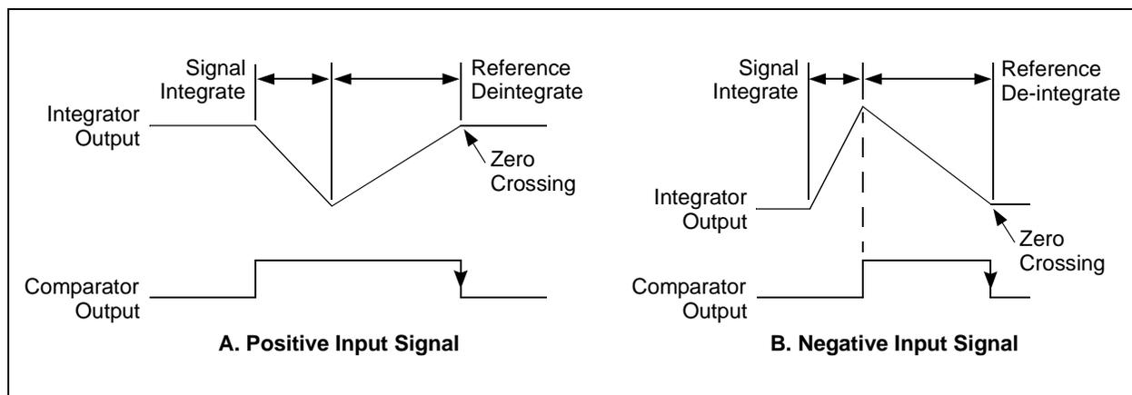
**FIGURE 6-1:** Comparator Output.
