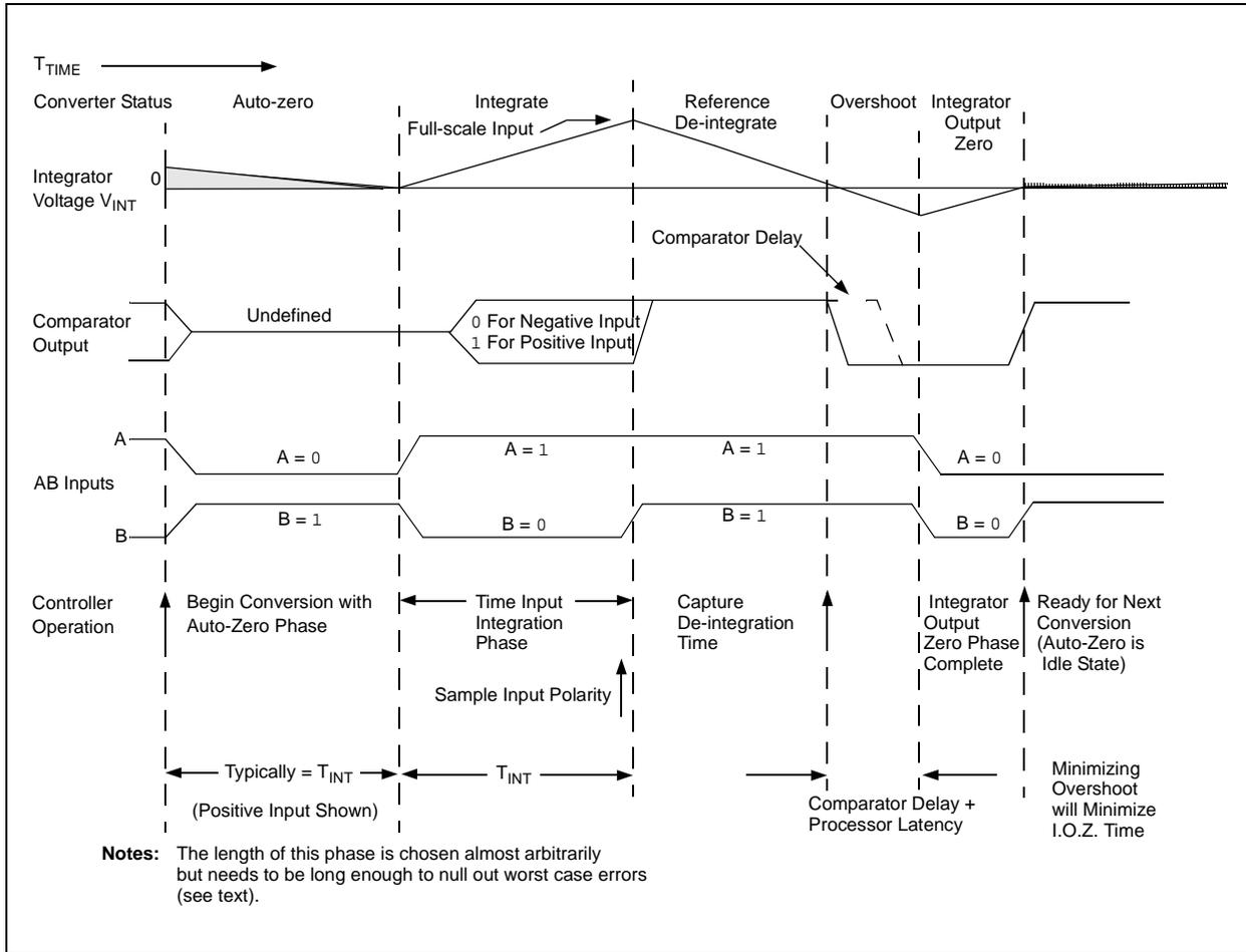
**FIGURE 5-1:** Typical Dual Slope A/D Converter System Timing.
