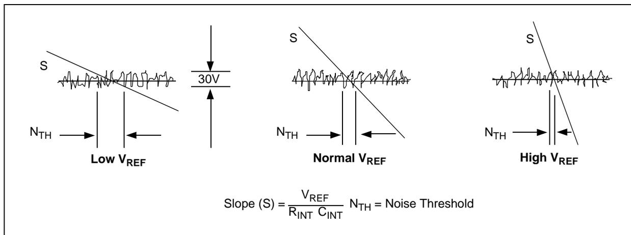
**FIGURE 8-1:** Noise Threshold.
