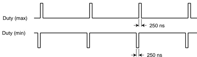
The voltage applied to the motor is duty 100% because of the storage time of the drive circuit even if the duty is 99%.
