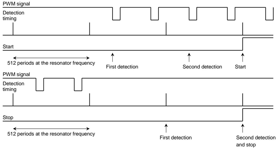
Note: Take sufficient care for noise on PWM signal input pin.
