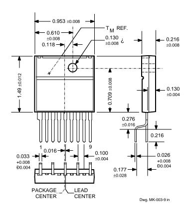
NOTE: Exact body and lead configuration at vendorÕs option within limits shown.
