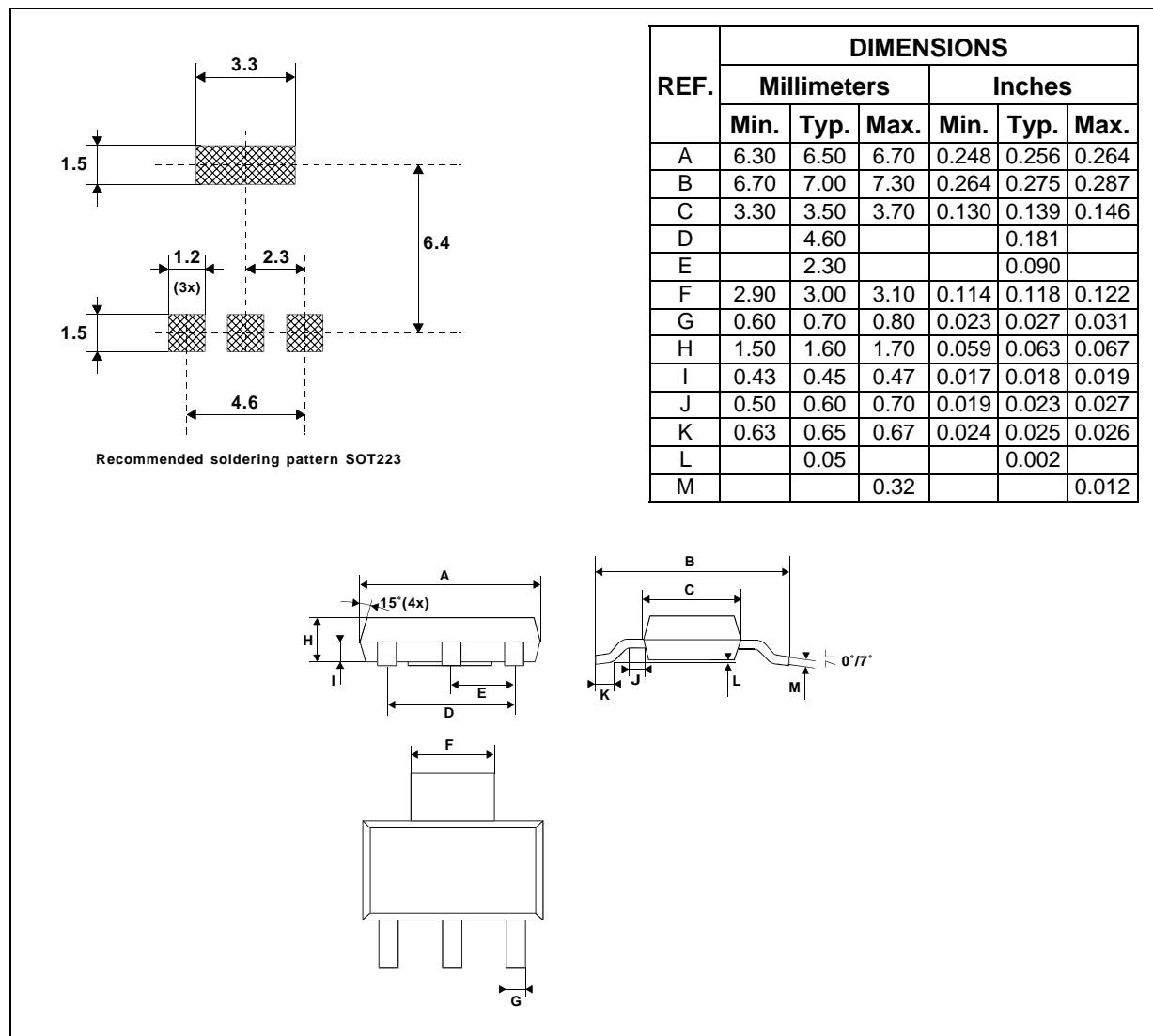
The technical drawing illustrates the physical dimensions and soldering pattern for the SOT223 package. It includes a top view showing lead spacing (4.6), lead height (1.5), and body width (6.4). A cross-sectional view shows lead thickness (A=6.30mm), lead height (H=1.5mm), and lead pitch (D=3.3mm). The recommended soldering pattern is also shown.
