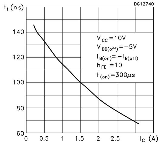
Switching Times Resistive Load
