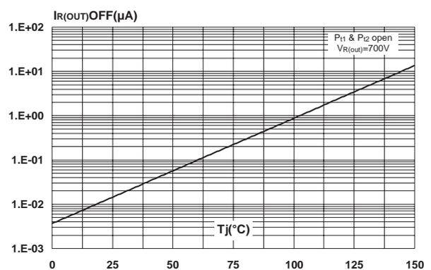
**Fig. 5-2:** Reverse current versus junction temperature with driver current (typical values).
